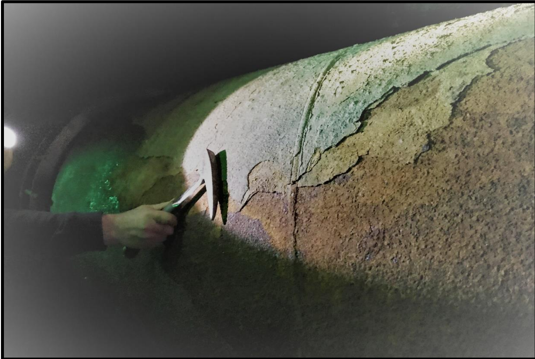
Photo 3. 48-inch diameter welded steel pipe, showing corrosion and iron oxide layers.
