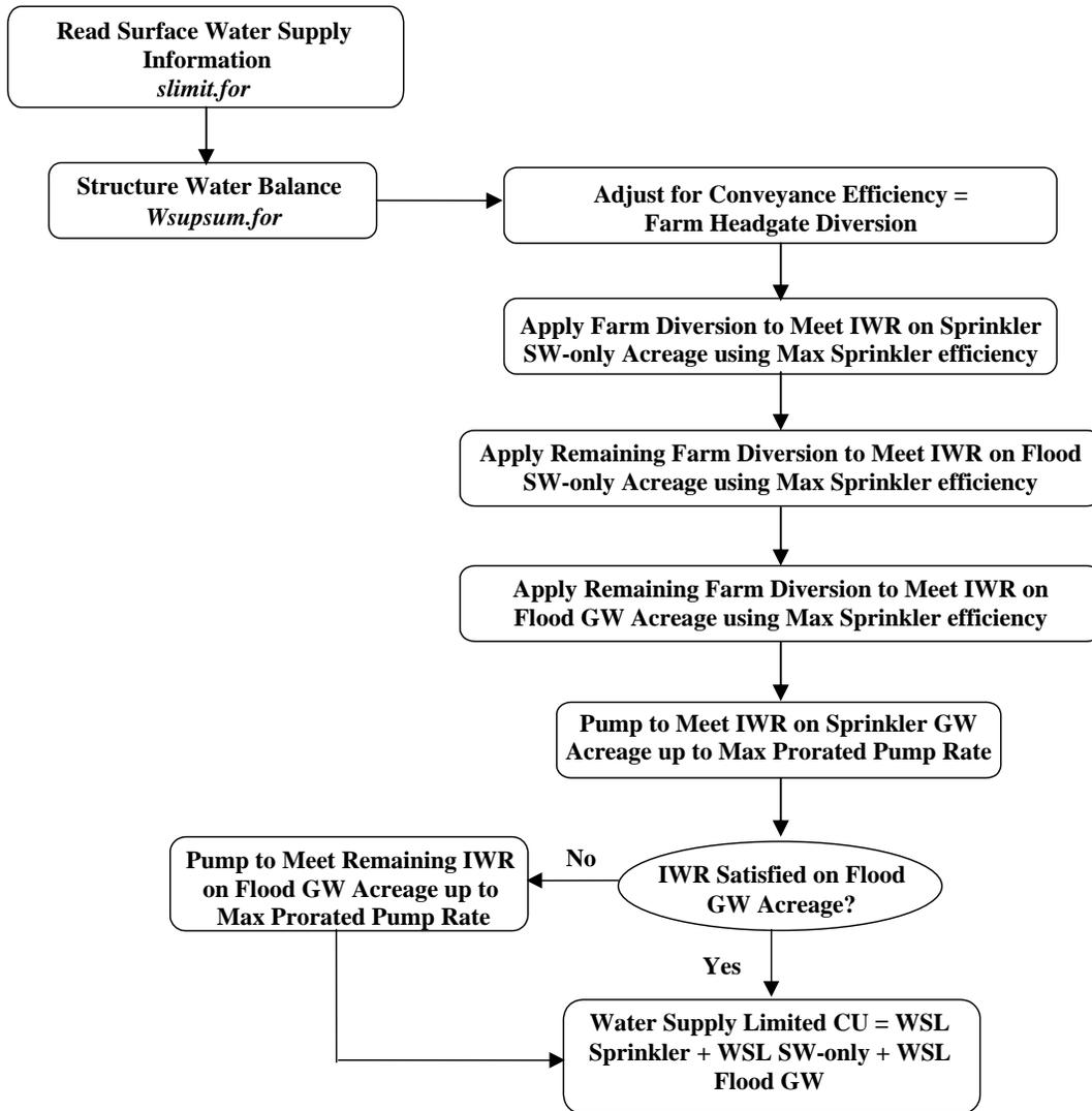
**Figure B-7 – Structure Water Balance Procedure Ground Water Available gmode = 1 - Maximize Supply Approach**
