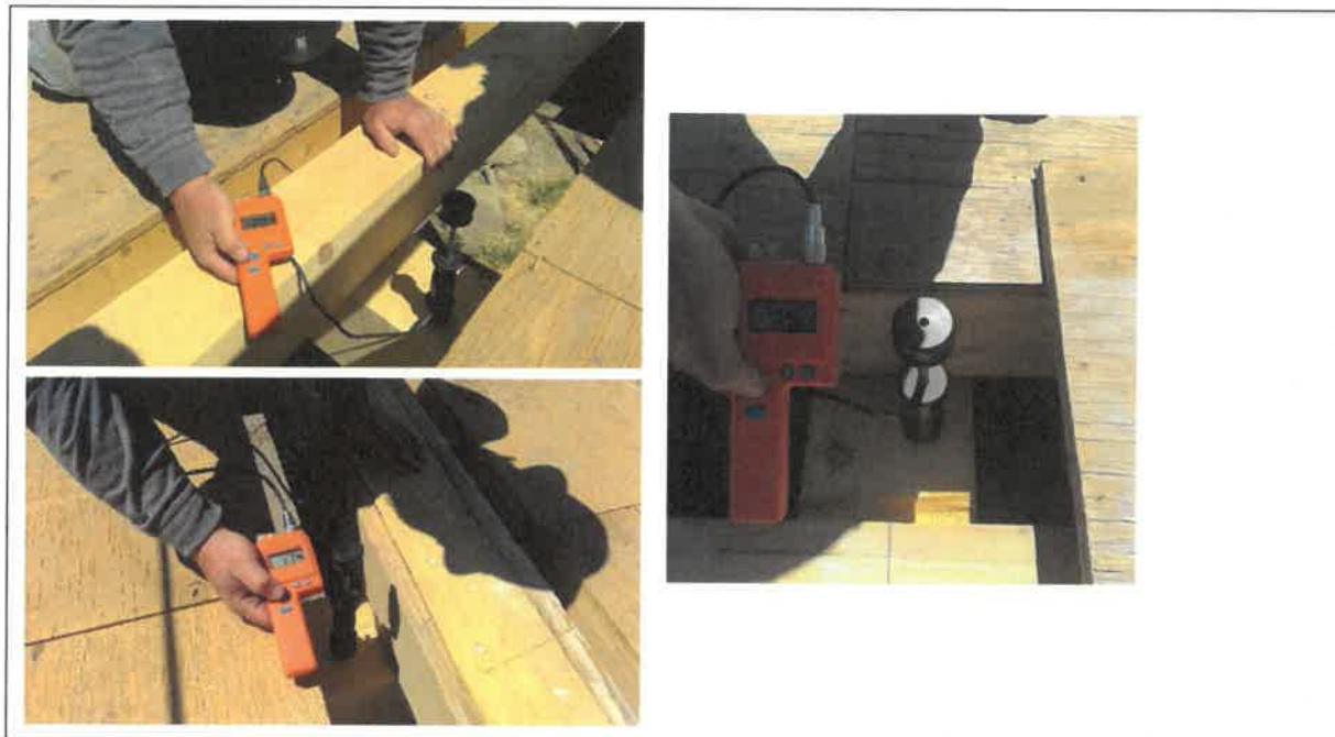
Figure 8. Moisture readings at stringers. Moisture content varies from approximately 17% to 20%.
