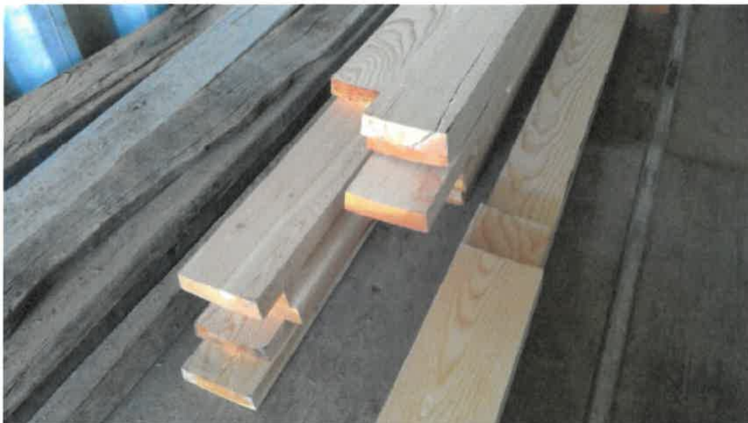
Figure 4. An example of a new stave with large end split.
