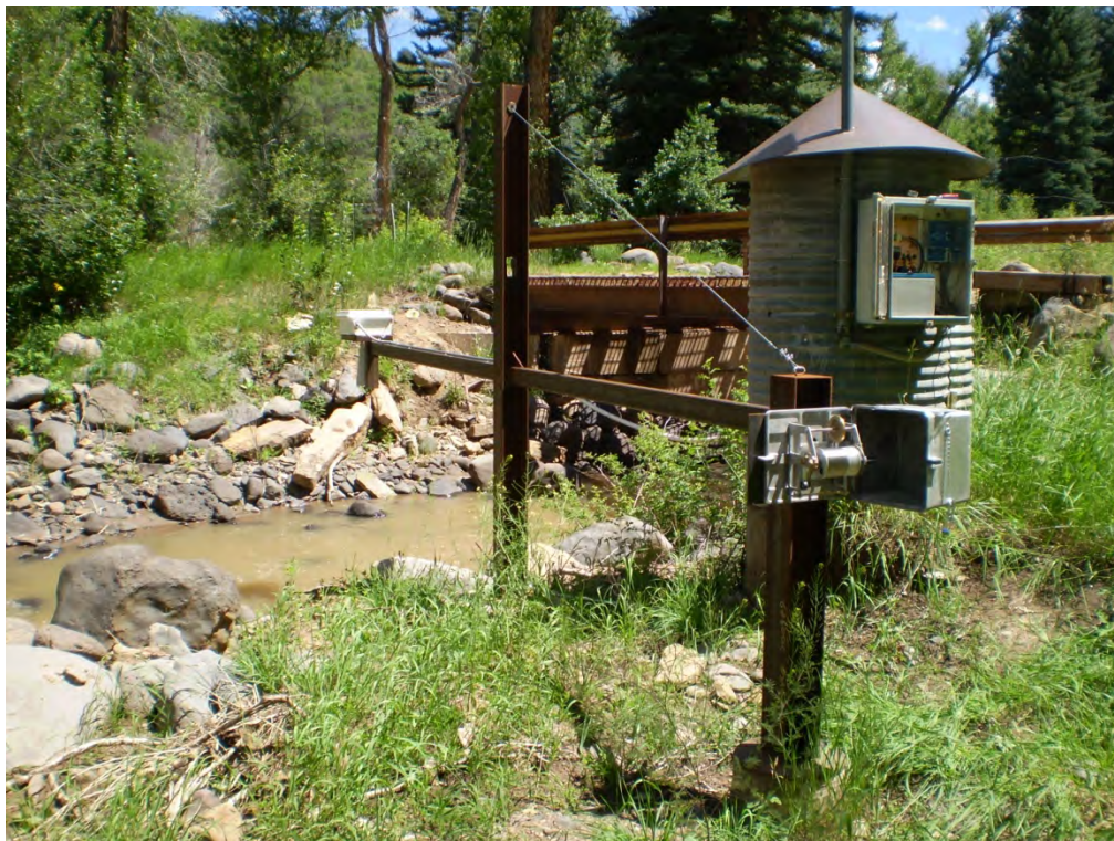
North Fork Gunnison River - New Radar Sensor Installation (Note these installations are more cost efficient as they require significantly less infrastructure than a typical stilling well and shelter)
