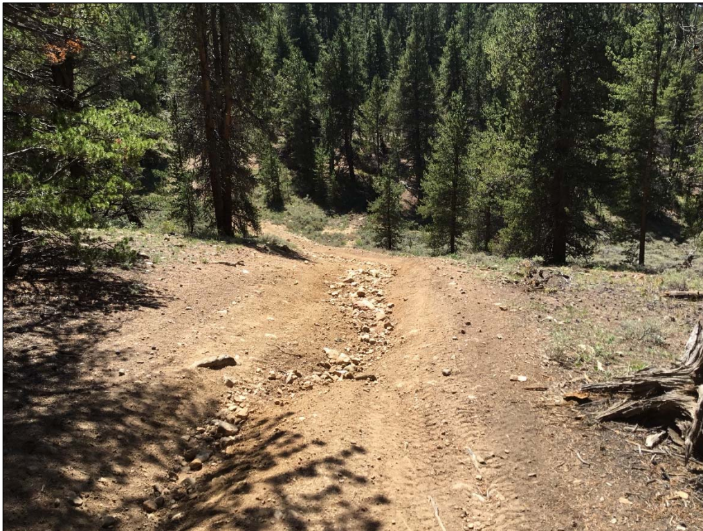
Image 6. Another example of an illegal route in the project area that needs to be closed and brought back to a natural state. We would use heavy equipment and rip the road and build water bars to prevent further erosion. There is a stream at the bottom of this hill and sediment is going directly into the stream.
