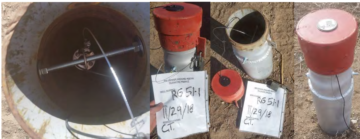
Picture 51, 52, 53, 54: RG 51-1 telemetry well site installation. Pictures 51- 53 show installation at the beginning of the month. Picture 54 shows evidence of vandalism of the well's antenna, the removal of the wire from the antenna piece. RG 51-1 is approximately 1/4 mile east on North County Road 3 East, near County Road 3 N in Alamosa County.
