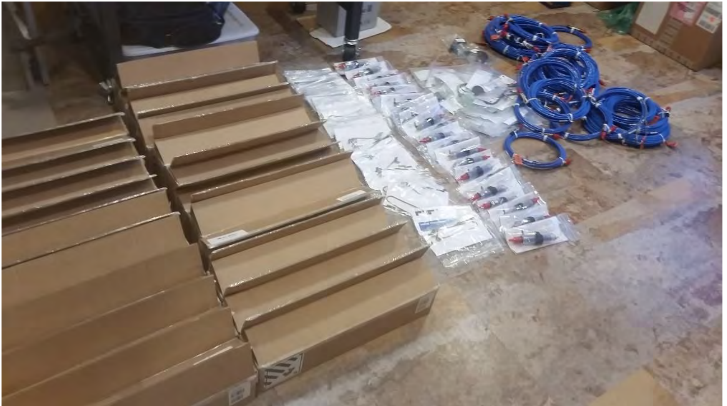
Picture 1: 22 telemetry setups in the office ready for installation. Telemetry tubes in boxes, blue coils of cables, hangar and desiccant kits.
