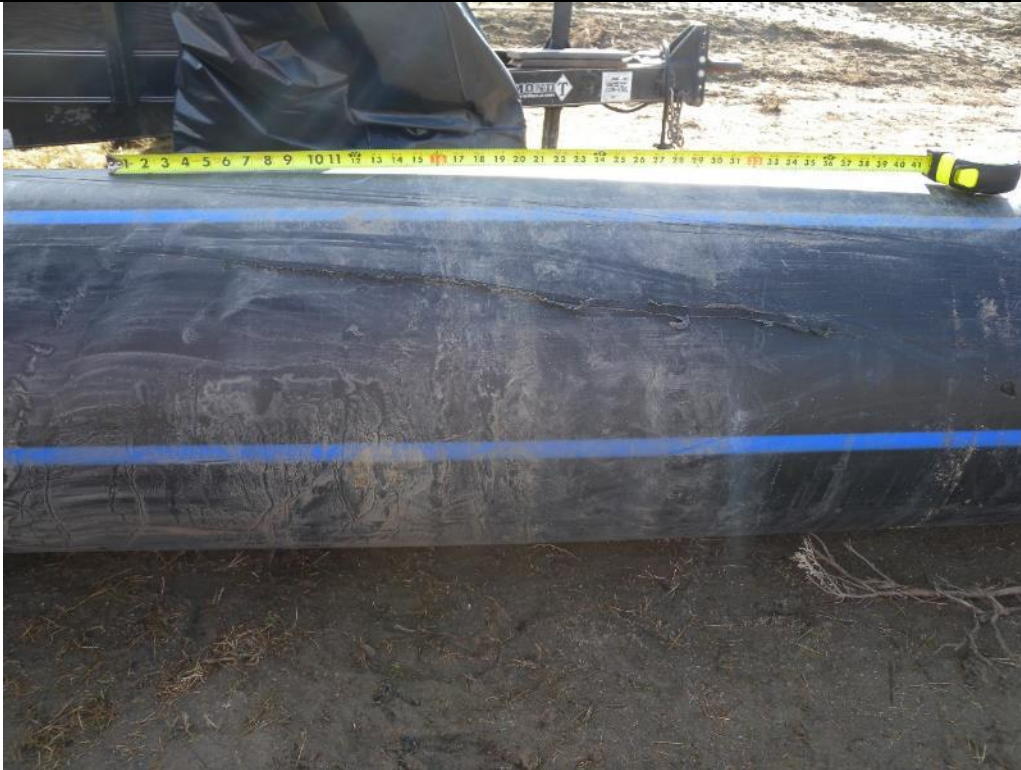
Photo 65. View of the test section after being pulled into the host pipe approximately 85 to 90 feet with no centralizers or grout tubes attached. Note the scratches around the exterior of the pipe. This bare test pull was also abandoned because the test section became stuck on an unknown obstacle approximately 90 feet up the host pipe from the downstream end. Sept. 29, 2017.
