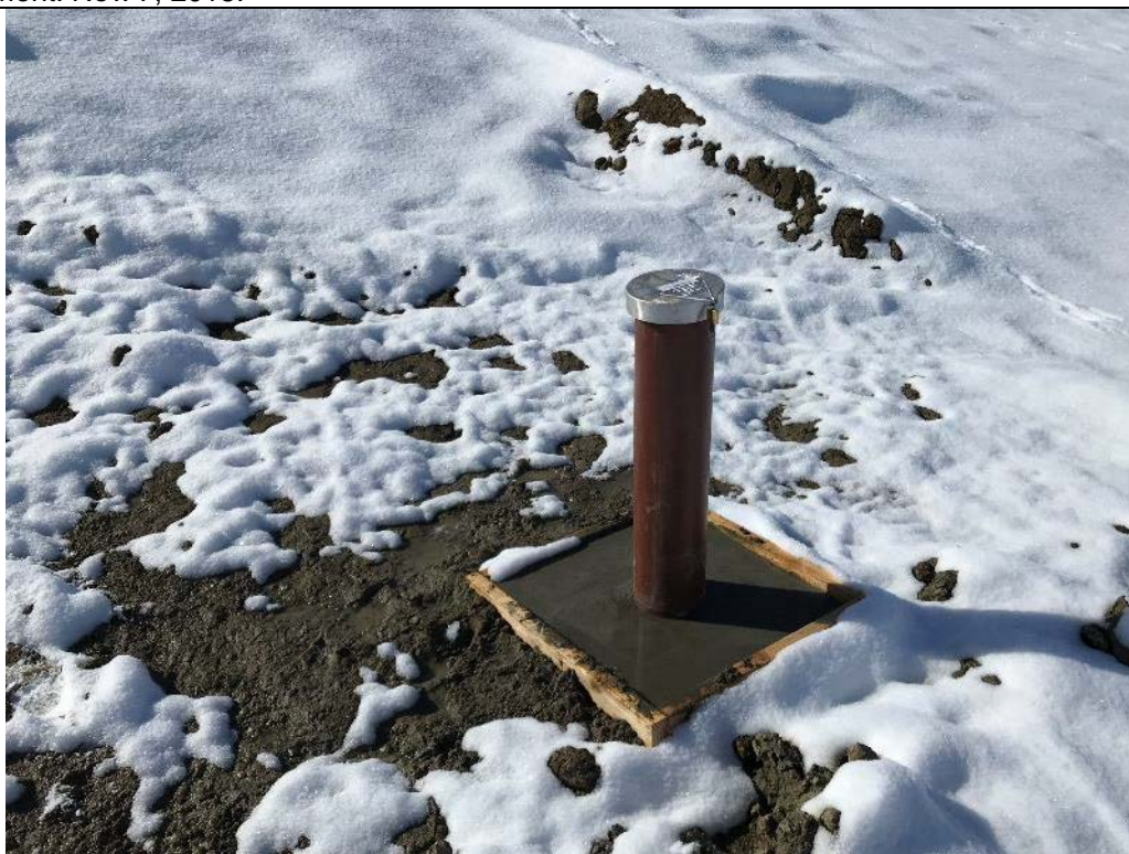
Photo 113. View looking down at the newly drilled replacement piezometer on the toe of the Main Dam, to the left of the outlet works. Nov. 7, 2018.
