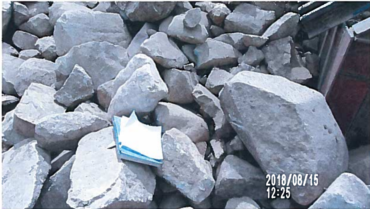
Picture showing riprap size, note clipboard for scale
