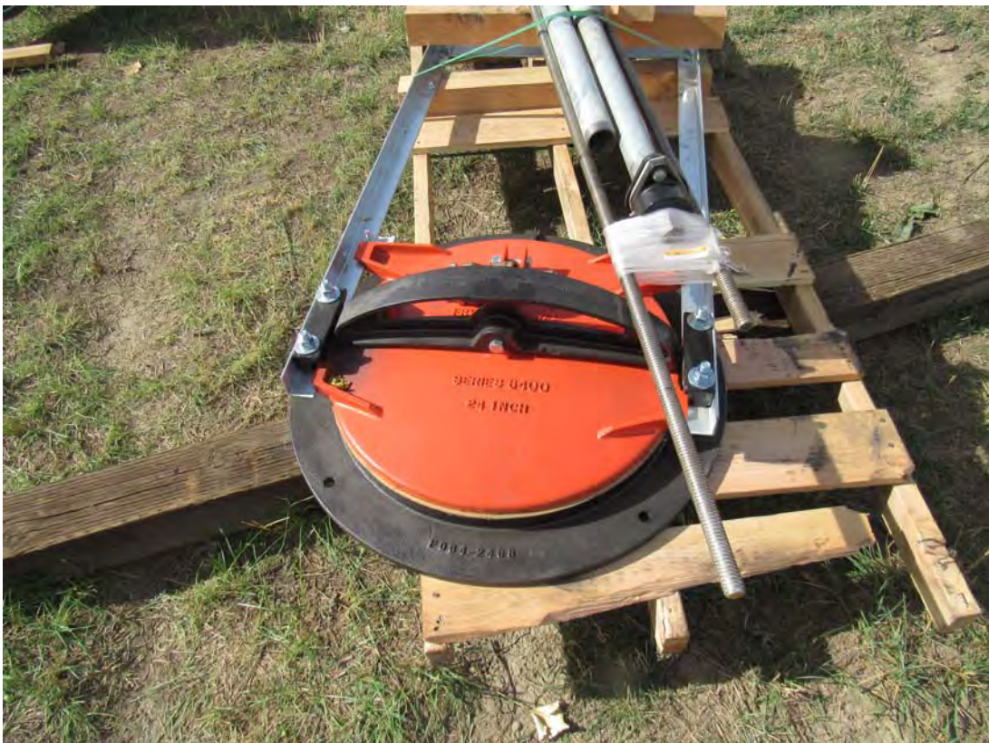
Photo 08 (10-24-2017) 24-inch heavy duty slide gate
