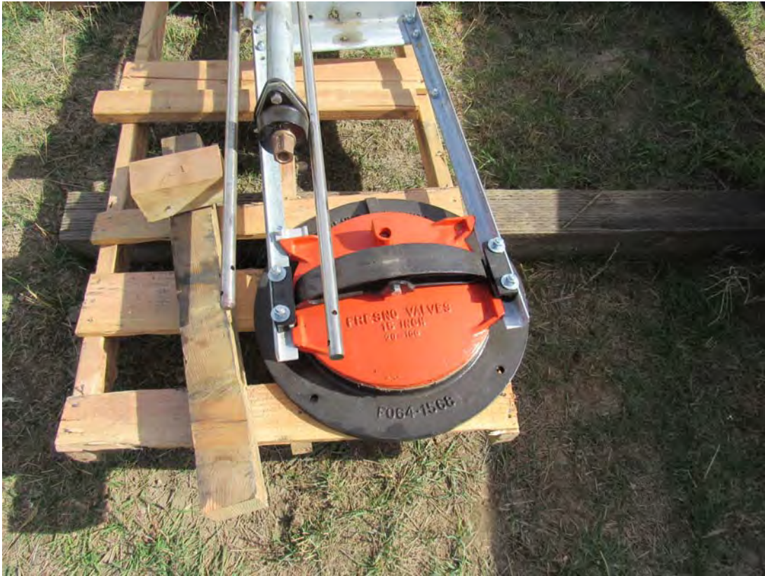
Photo 07 (10-24-2017) 15-inch heavy duty slide gate
