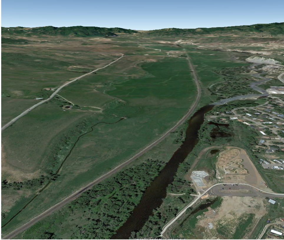
Figure 9. Floodplain and riparian area cut off by railroad line.
