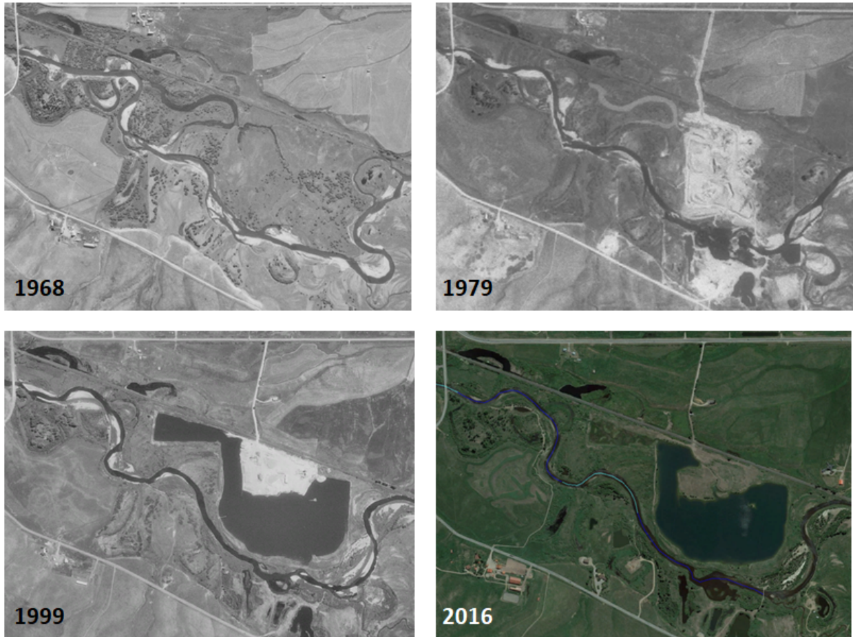
Figure 10. Aggregate mining was an invasive land use on the Chuck Lewis SWA segment in the 1970s through 1990s. Mined lands were reclaimed as gravel pit ponds and depressional wetland, but the channelized river form and floodplain levees remain.
