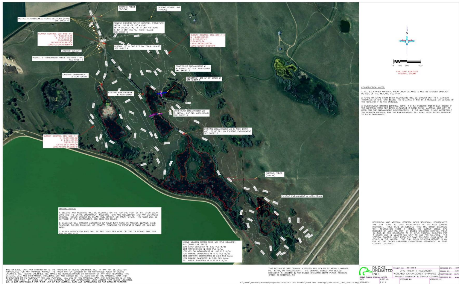
Figure 12. Final design plan set, page 2, for DPG Prewitt (CO-222-3). The project enhanced 107 acres of emergent wetlands near Merino, Colorado. Plan set depicts location of embankments and water control structures.
