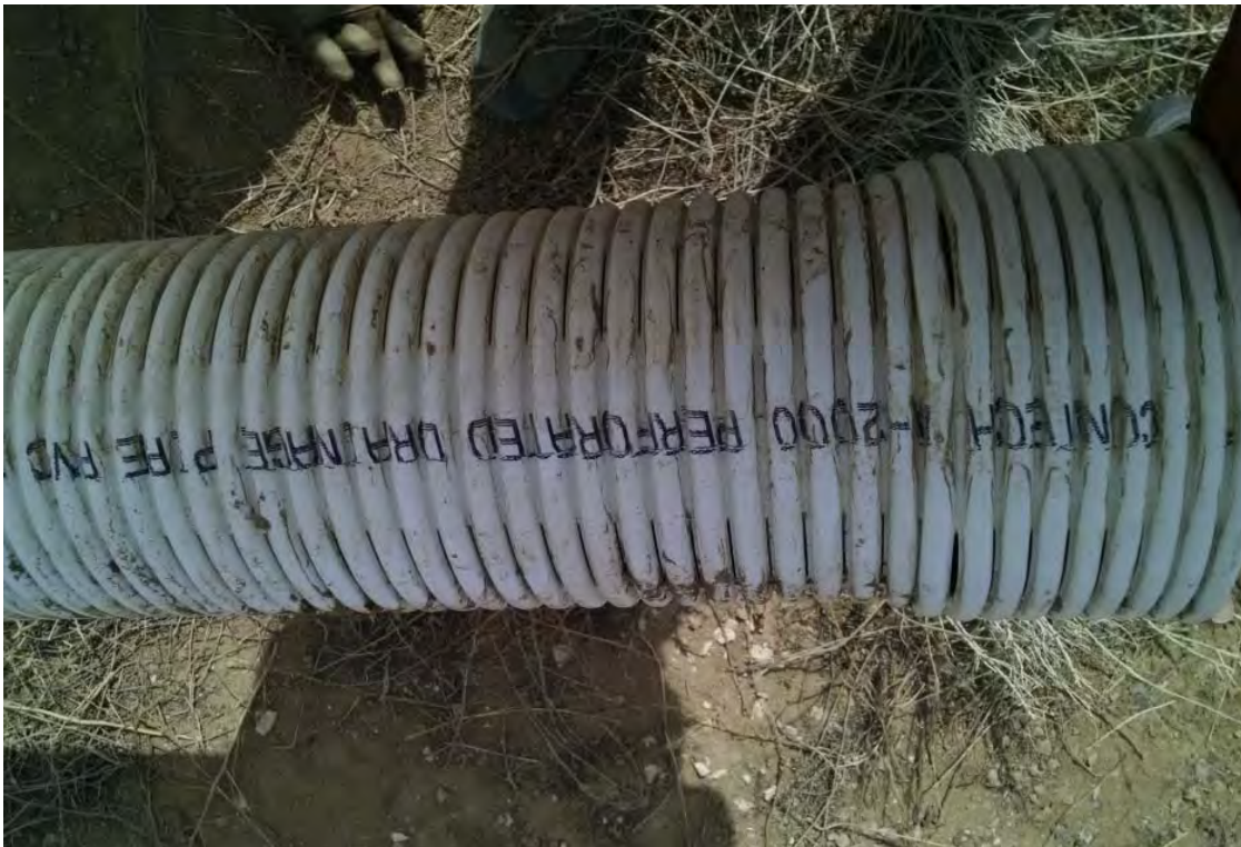
Photo 8: View of the bottom of new 6-inch-diameter slotted PVC drain pipe (Contech A2000). March 25, 2016.
