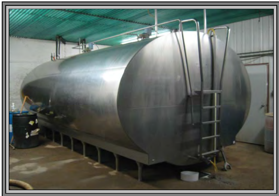
Milk Storage Tank
