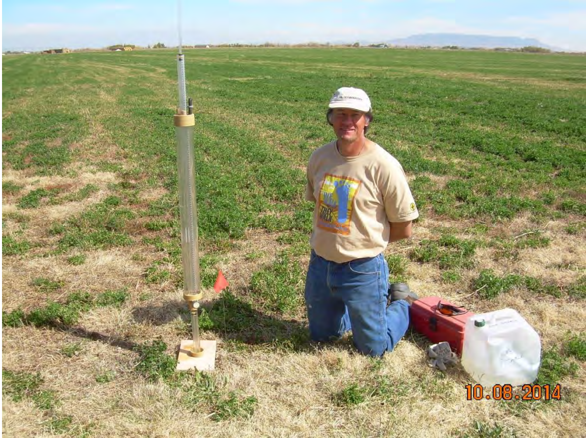
Figure 9: Measuring soil permeability. San Antonio test site. October, 2014.
