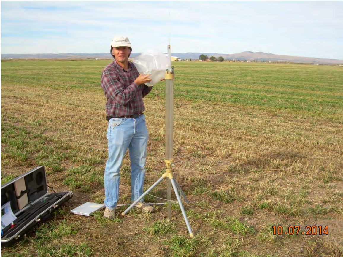
Figure 8: Filling Guelph permeameter for soil permeability measurement. San Antonio test site. October, 2014.
