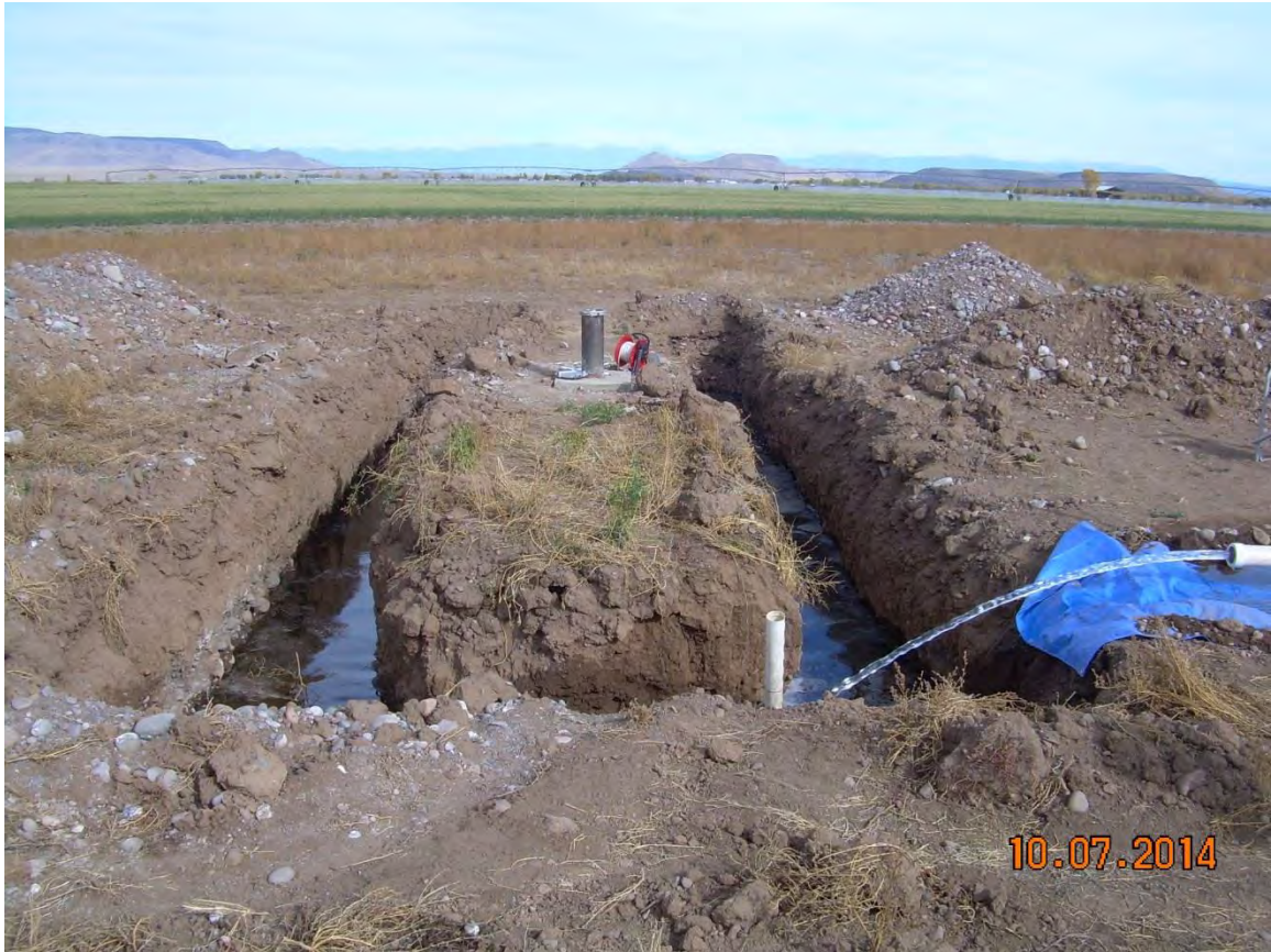
Figure 11: Infiltration rate testing. Conejos West test site. October, 2014.
