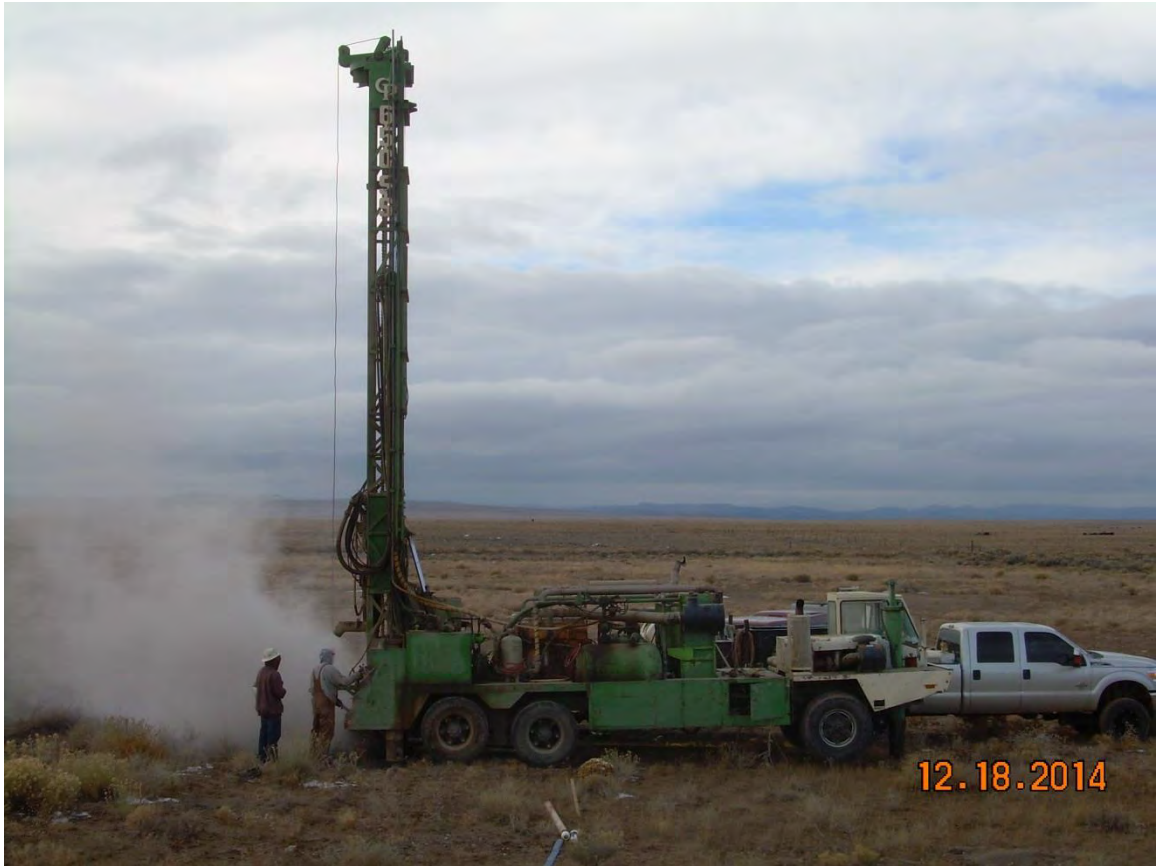
Figure 4: Drilling shallow piezometer at Bountiful West test site. December, 2014.
