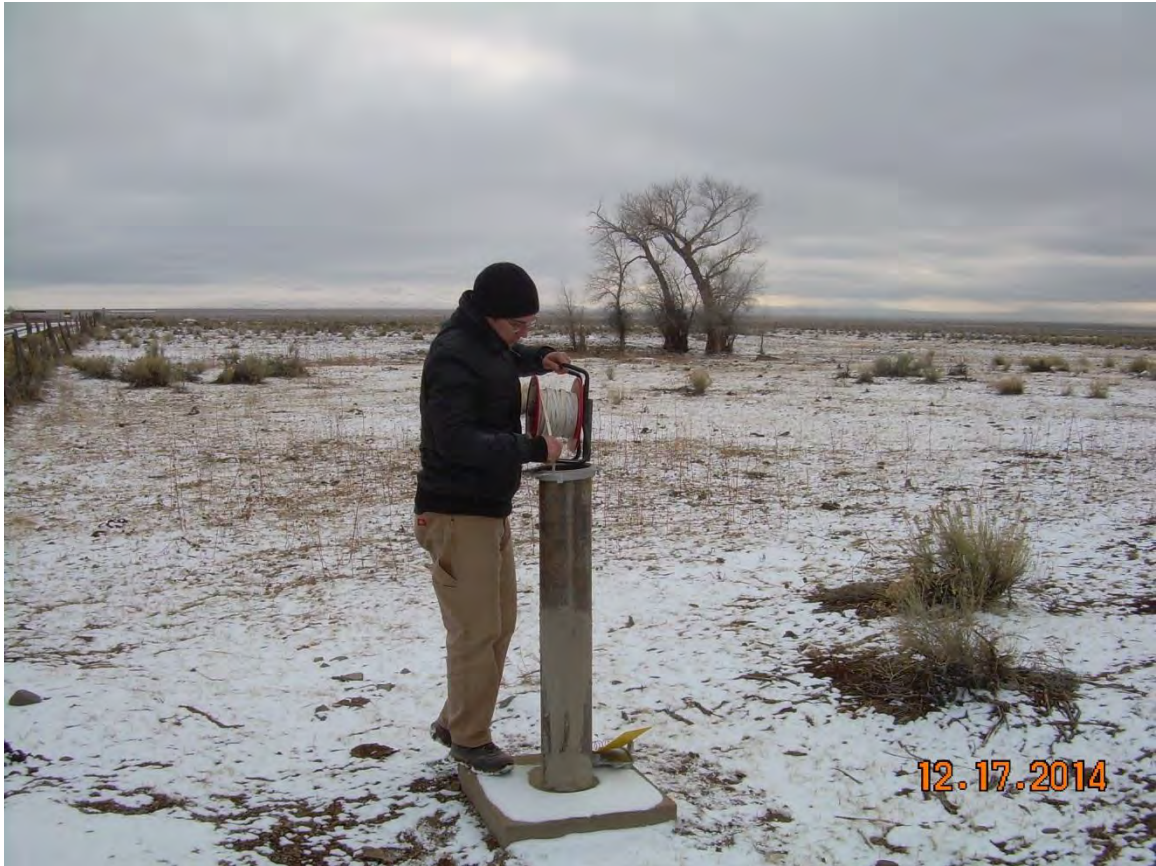
Figure 6: Measuring water level at Punche North piezometer. December, 2014.
