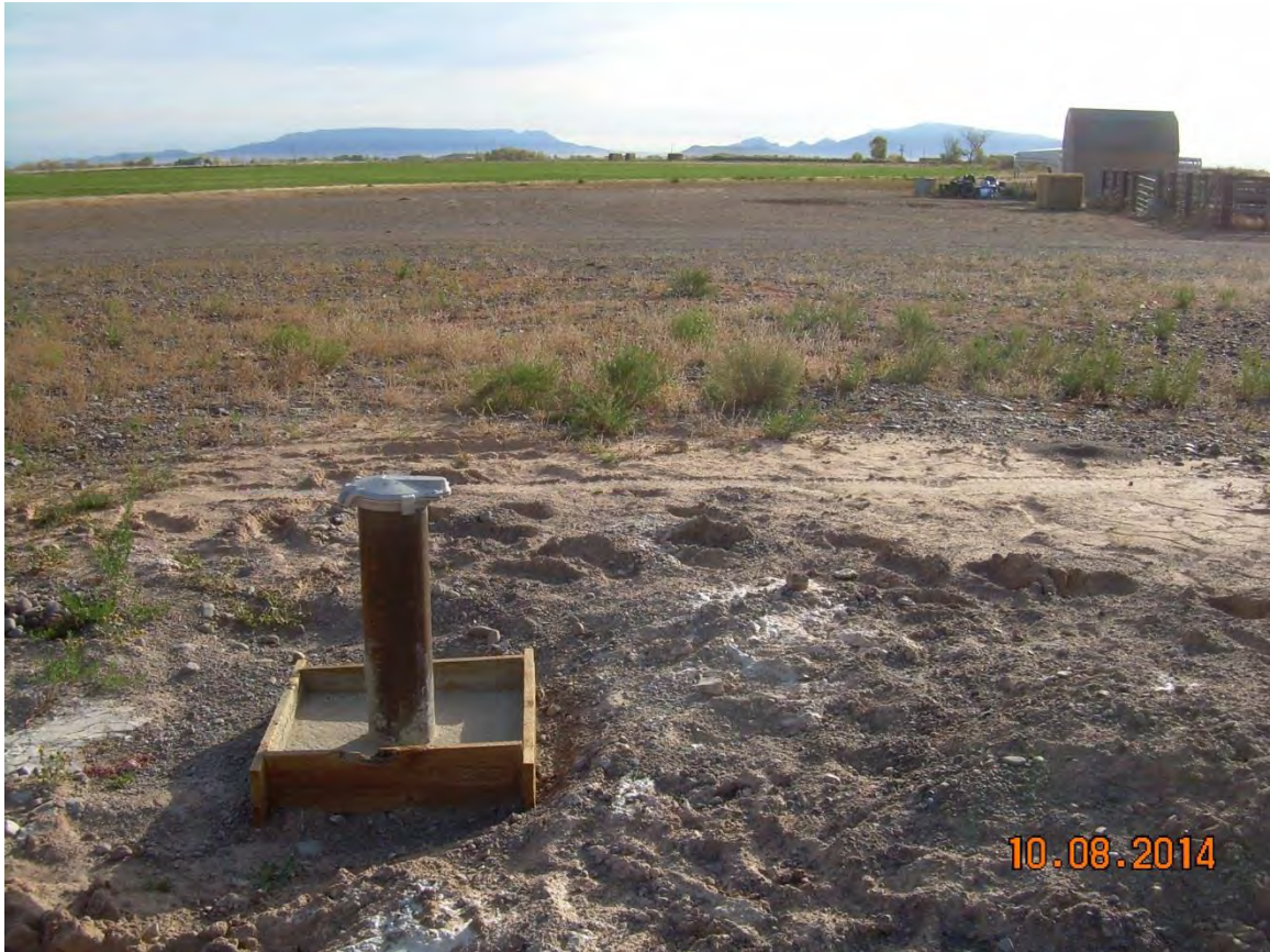
Figure 5: Conejos West Site: wellhead completion at deep piezometer.
