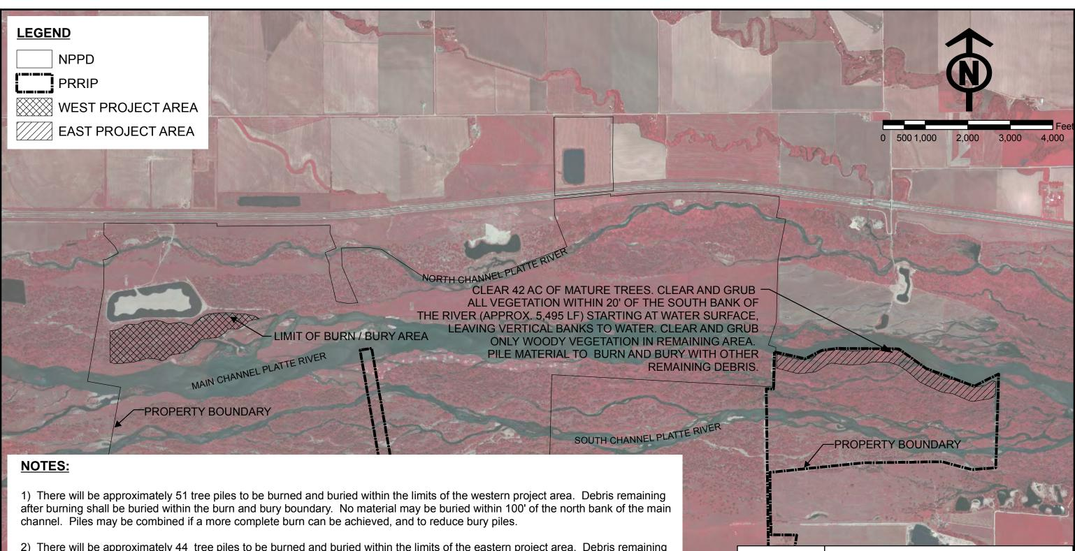
2) There will be approximately 44 tree piles to be burned and buried within the limits of the eastern project area. Debris remaining after burning shall be buried within the burn and bury boundary. No material may be buried within 100' of the south bank of the main channel. Piles may be combined if a more complete burn can be achieved, and to reduce bury piles.
