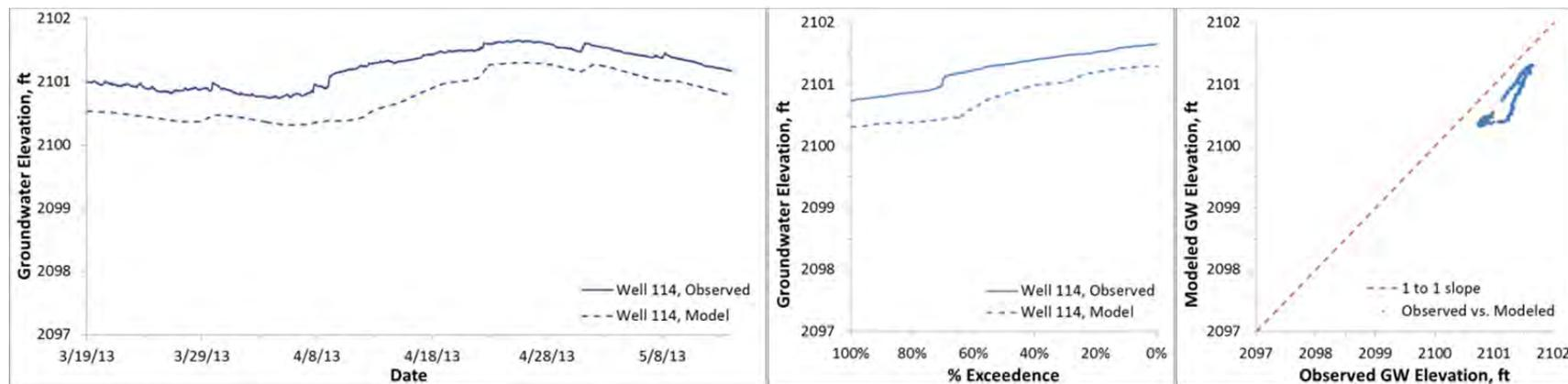
Figure C9. Modeled and observed heads, Fox well 114 (ground surface elevation 2105.6 ft)
