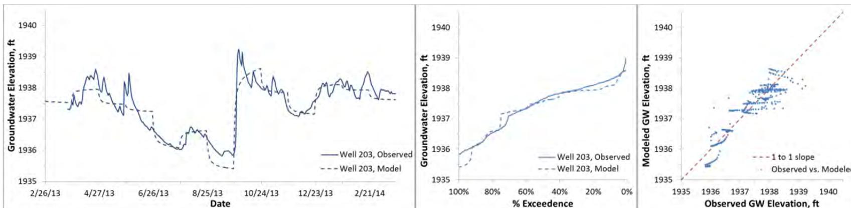
Figure B19. Modeled and observed heads 2013-2014, Binfield well 203 (ground surface elevation 1939.4 ft)
