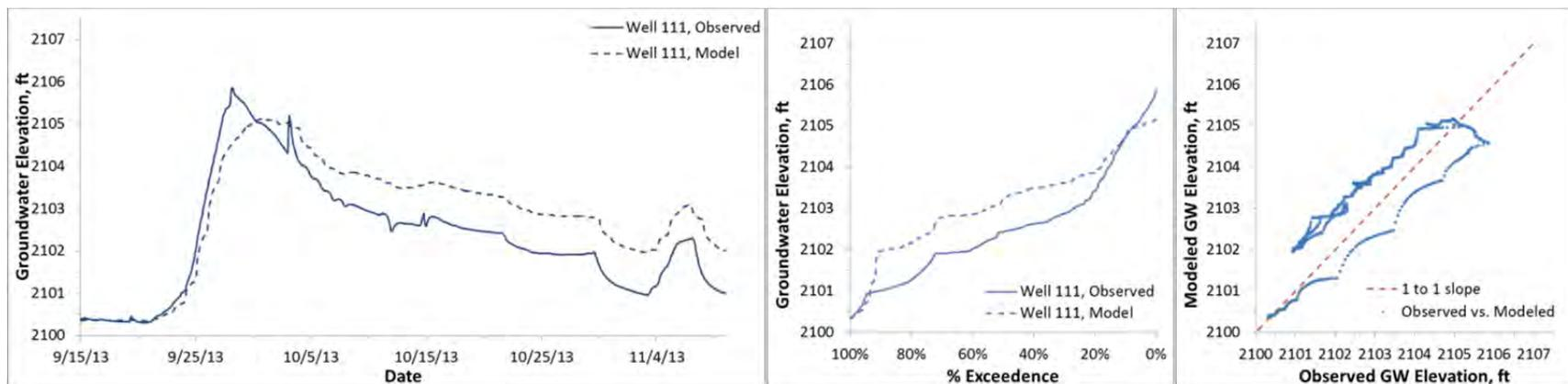
**Figure D13.** Modeled and observed heads, Fox well 111 (ground surface elevation 2107.9 ft)
