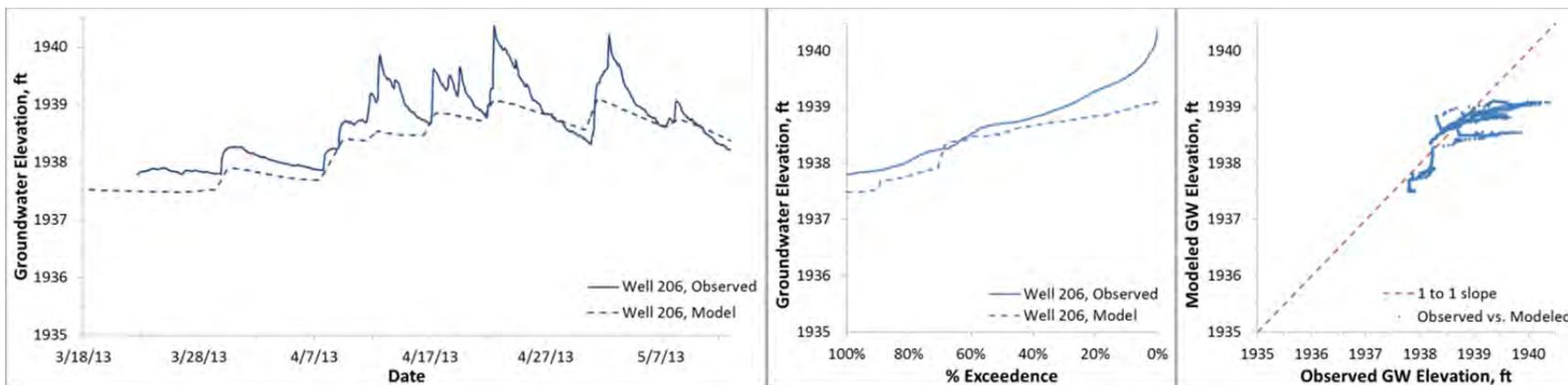
Figure C13. Modeled and observed heads, Binfield well 206 (ground surface elevation 1940.8 ft)
