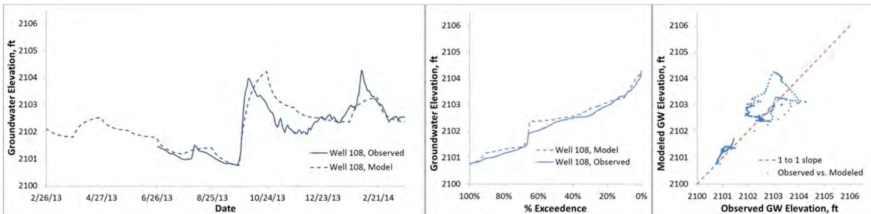
**Figure B10.** Modeled and observed heads 2013-2014, Fox well 108 (ground surface elevation 2110.5 ft)
