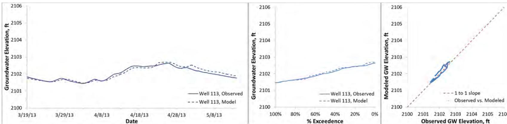
Figure C5. Modeled and observed heads, Fox well 113 (ground surface elevation 2107.6 ft)
