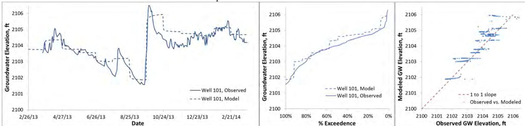
756 **Figure B1.** Modeled and observed heads 2013-2014, Fox well 101 (ground surface elevation 2110.1 ft)
