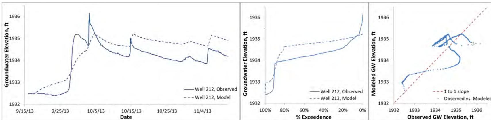
Figure D28. Modeled and observed heads, Binfield well 212 (ground surface elevation 1937.7 ft)
