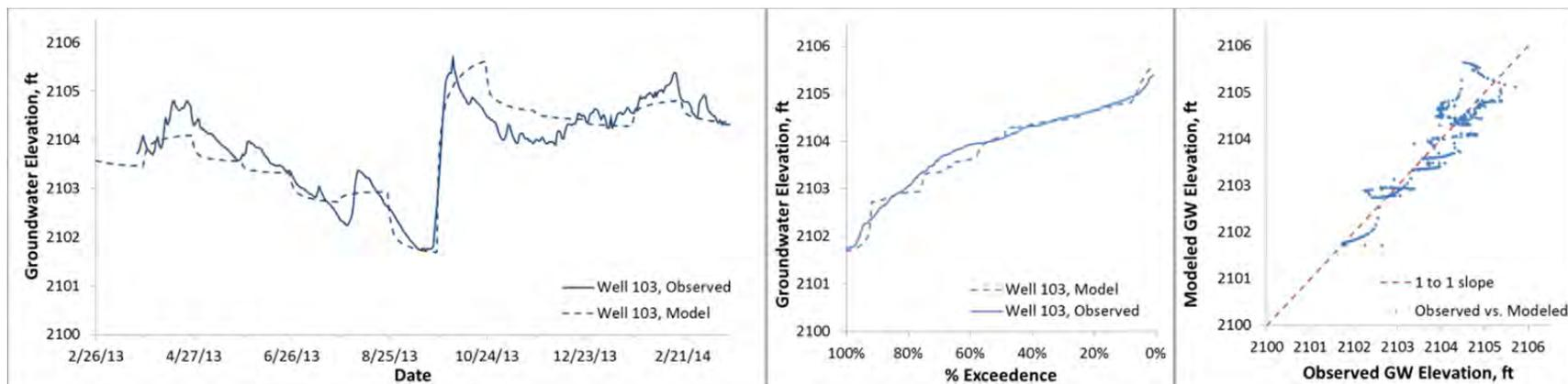
**Figure B3.** Modeled and observed heads 2013-2014, Fox well 103 (ground surface elevation 2110.3 ft)
