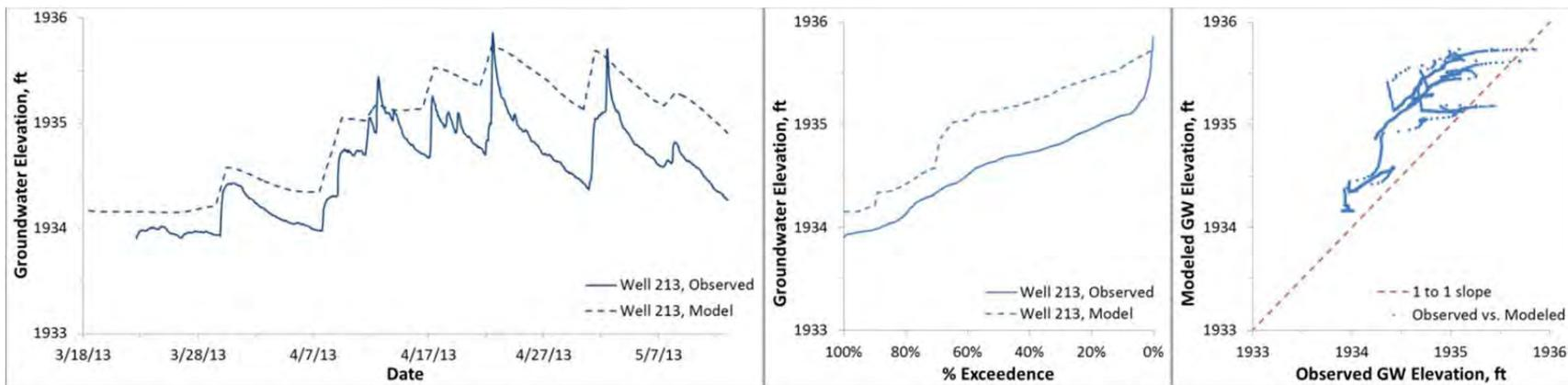
**Figure C16.** Modeled and observed heads, Binfield well 213 (ground surface elevation 1937.3 ft)
