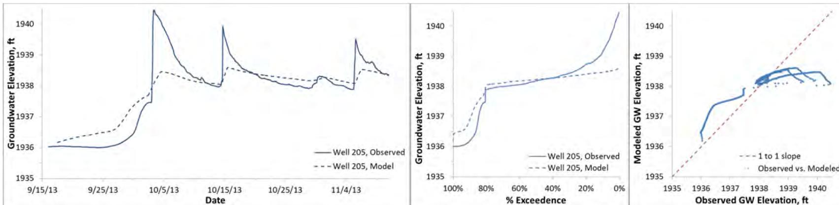
**Figure D21.** Modeled and observed heads, Binfield well 205 (ground surface elevation 1940.5 ft)
