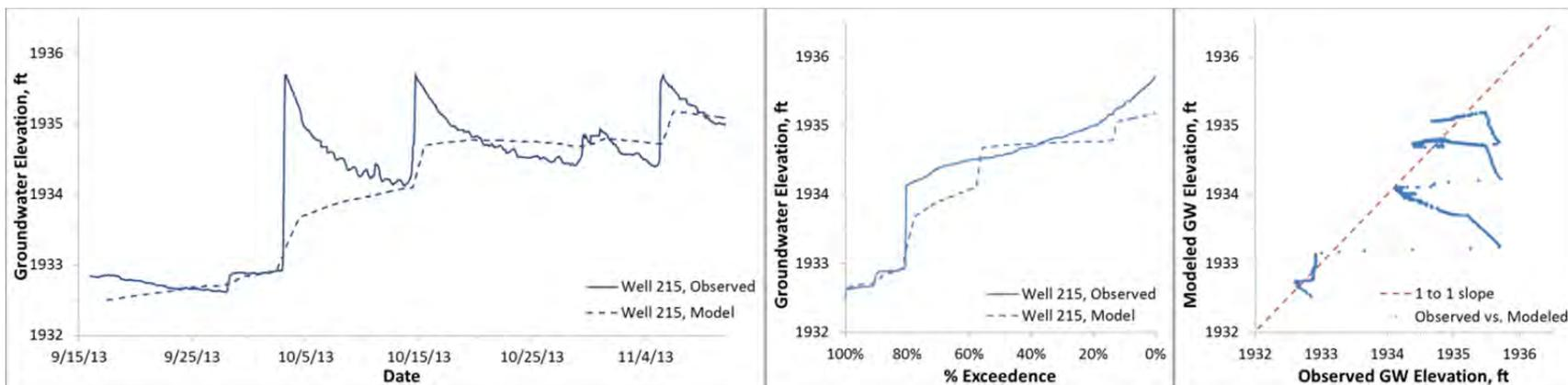
Figure D31. Modeled and observed heads, Binfield well 215 (ground surface elevation 1936.4 ft)
