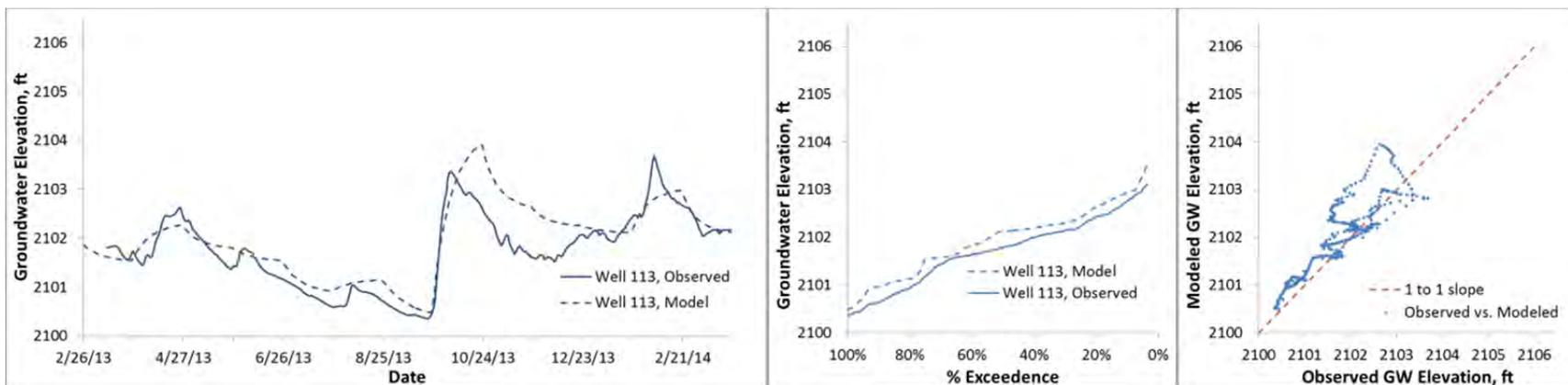
**Figure B9.** Modeled and observed heads 2013-2014, Fox well 113 (ground surface elevation 2107.6 ft)
