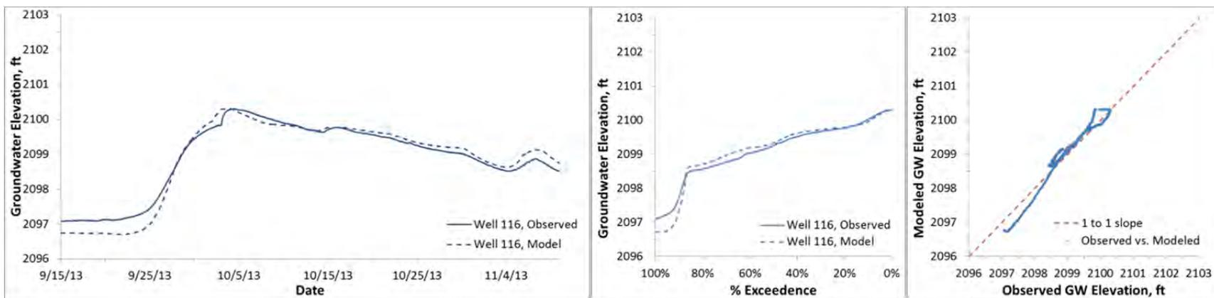
Figure D16. Modeled and observed heads, Fox well 116 (ground surface elevation 2105.0 ft)
