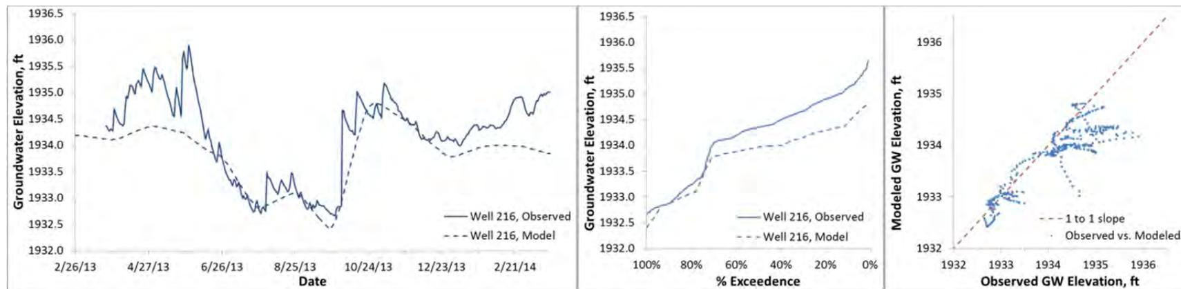
Figure B32. Modeled and observed head 2013-2014s, Binfield well 216 (ground surface elevation 1936.3 ft)
