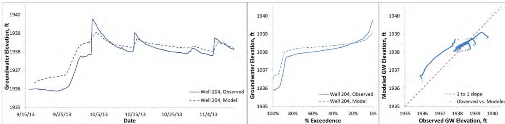
Figure D20. Modeled and observed heads, Binfield well 204 (ground surface elevation 1941.4 ft)
