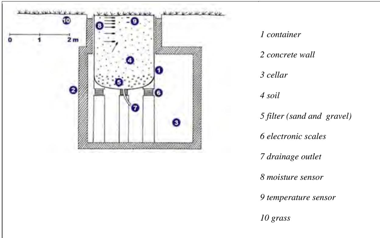
192 **Figure 4:** Weighing lysimeter cross section (image credit:
