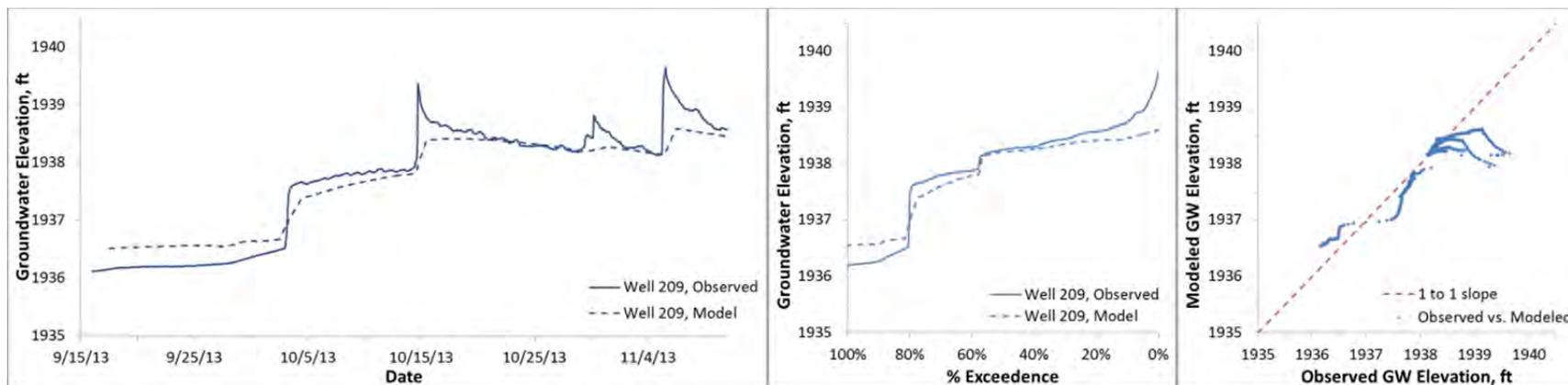
Figure D25. Modeled and observed heads, Binfield well 209 (ground surface elevation 1940.6 ft)
