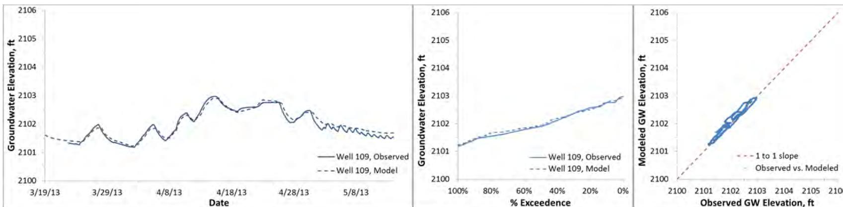
Figure C6. Modeled and observed heads, Fox well 109 (ground surface elevation 2108.1 ft)
