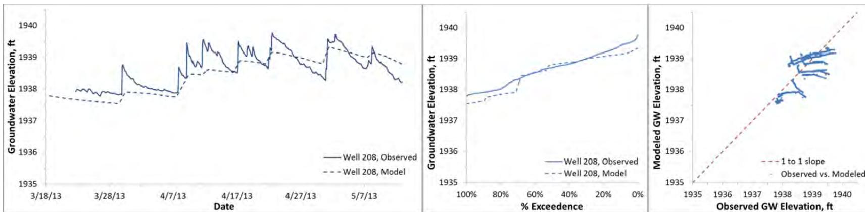
Figure C14. Modeled and observed heads, Binfield well 208 (ground surface elevation 1940.4 ft)
