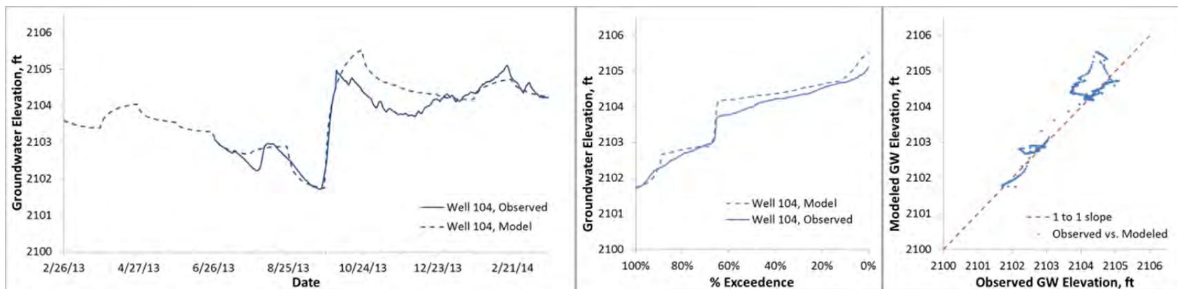
**Figure B4.** Modeled and observed heads 2013-2014, Fox well 104 (ground surface elevation 2107.1 ft)
