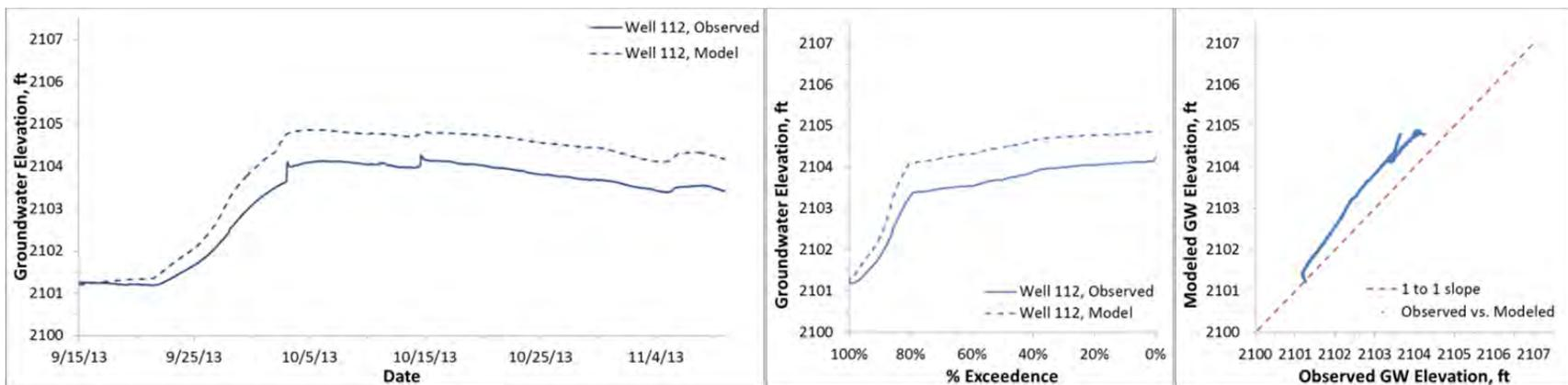
Figure D5. Modeled and observed heads, Fox well 112 (ground surface elevation 2107.4 ft)
