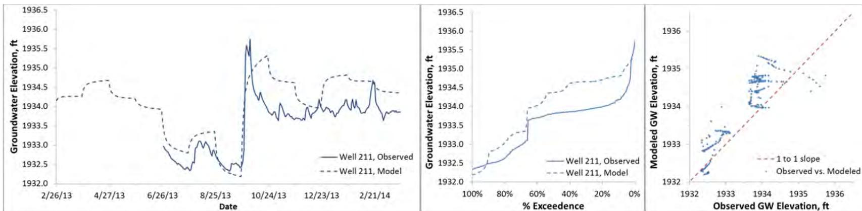
Figure B27. Modeled and observed heads 2013-2014, Binfield well 211 (ground surface elevation 1937.8 ft)
