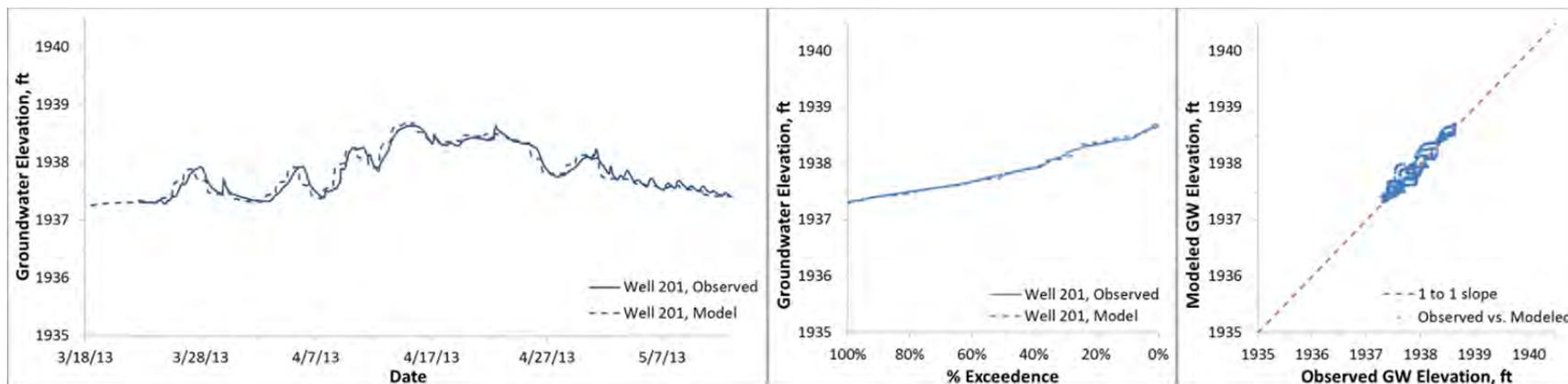
Figure C11. Modeled and observed heads, Binfield well 201 (ground surface elevation 1939.2 ft)
