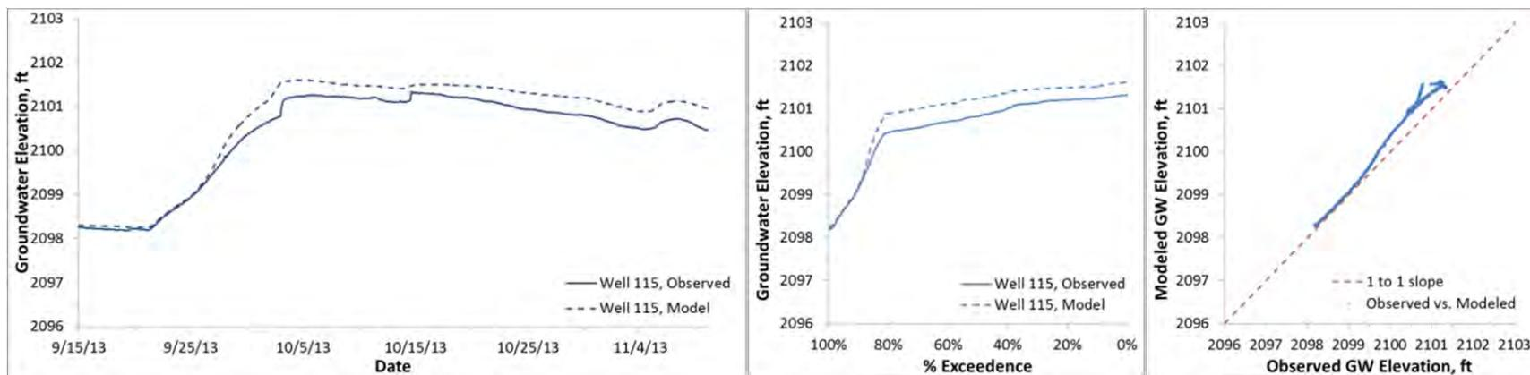
**Figure D14.** Modeled and observed heads, Fox well 115 (ground surface elevation 2105.9 ft)
