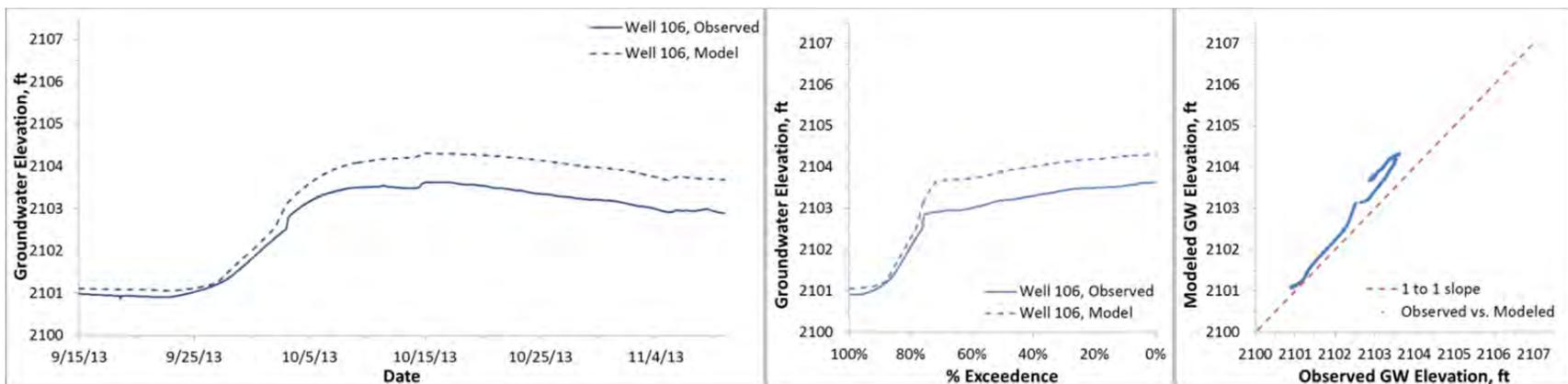
Figure D7. Modeled and observed heads, Fox well 106 (ground surface elevation 2107.7 ft)
