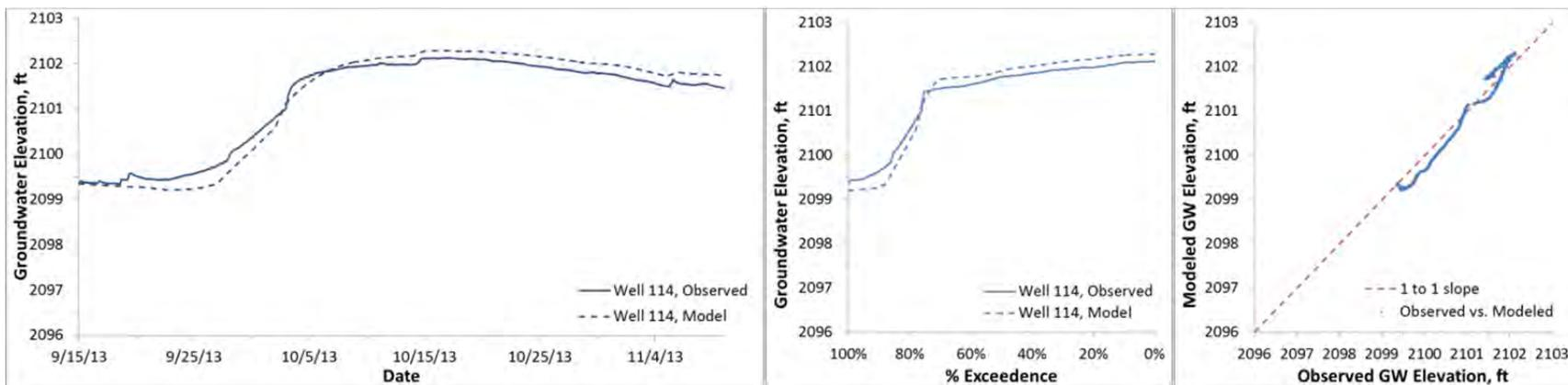
Figure D15. Modeled and observed heads, Fox well 114 (ground surface elevation 2105.6 ft)
