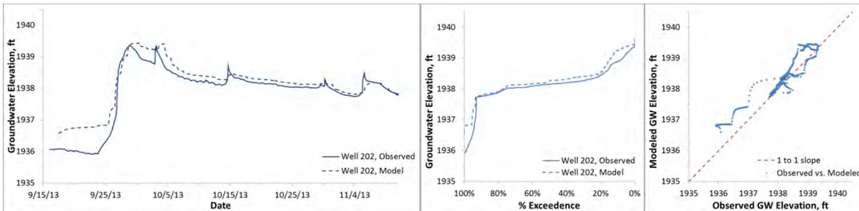
Figure D18. Modeled and observed heads, Binfield well 202 (ground surface elevation 1940.2 ft)
