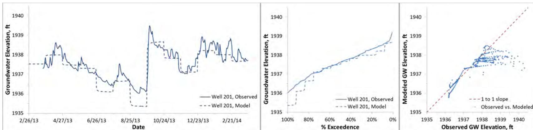
**Figure B17.** Modeled and observed heads 2013-2014, Binfield well 201 (ground surface elevation 1939.2 ft)
