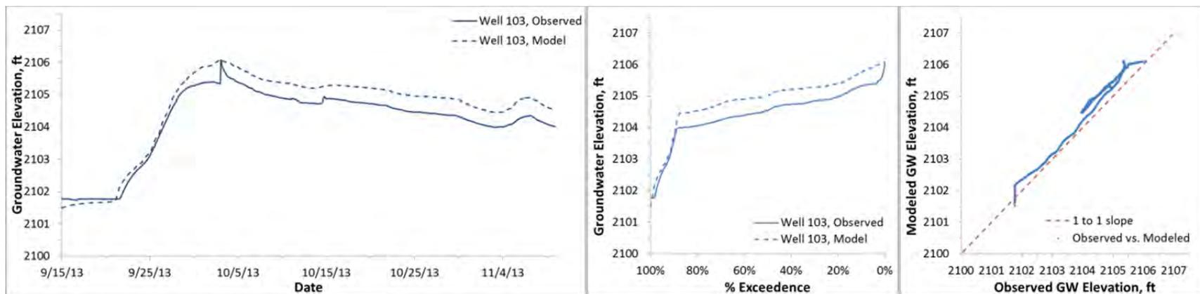
Figure D3. Modeled and observed heads, Fox well 103 (ground surface elevation 2110.3 ft)
