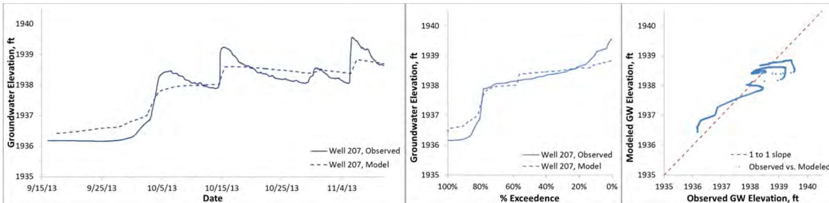
Figure D23. Modeled and observed heads, Binfield well 207 (ground surface elevation 1941.8 ft)
