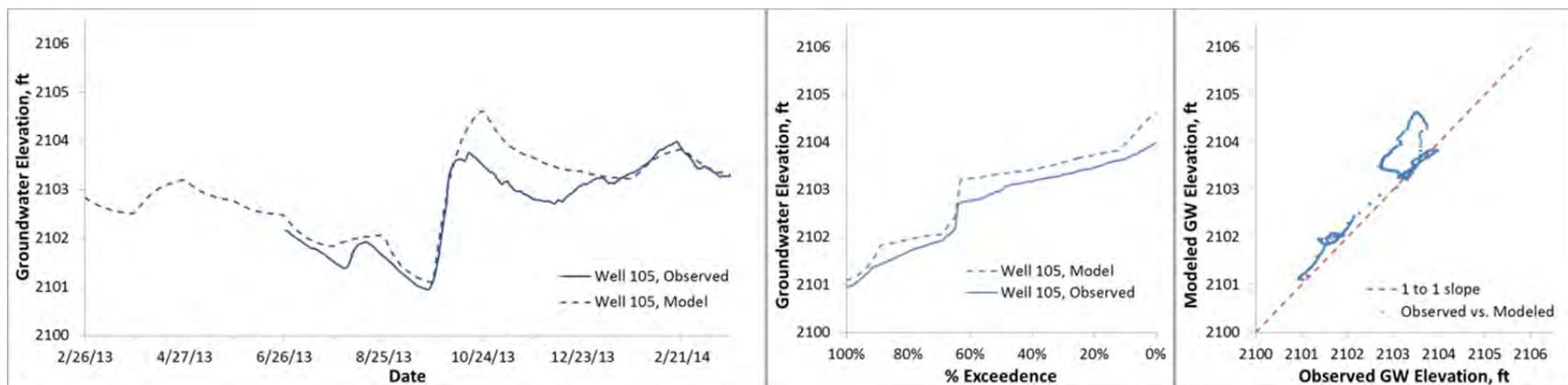
**Figure B6.** Modeled and observed heads 2013-2014, Fox well 105 (ground surface elevation 2107.7 ft)
