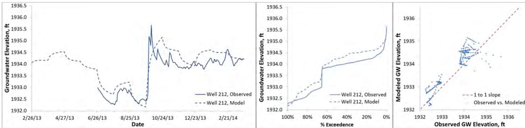
Figure B28. Modeled and observed heads 2013-2014, Binfield well 212 (ground surface elevation 1937.7 ft)
