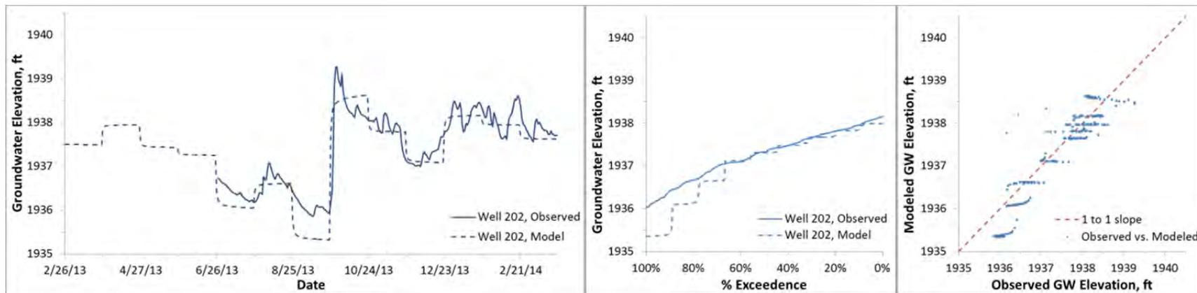
**Figure B18.** Modeled and observed heads 2013-2014, Binfield well 202 (ground surface elevation 1940.2 ft)
