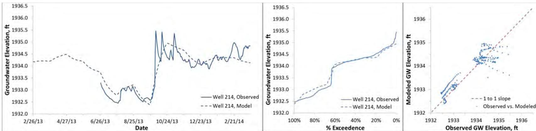
Figure B30. Modeled and observed heads 2013-2014, Binfield well 214 (ground surface elevation 1936.7 ft)
