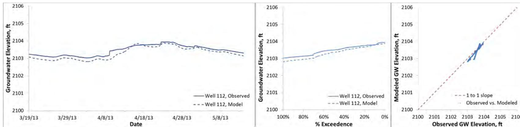
Figure C3. Modeled and observed heads, Fox well 112 (ground surface elevation 2107.4 ft)
