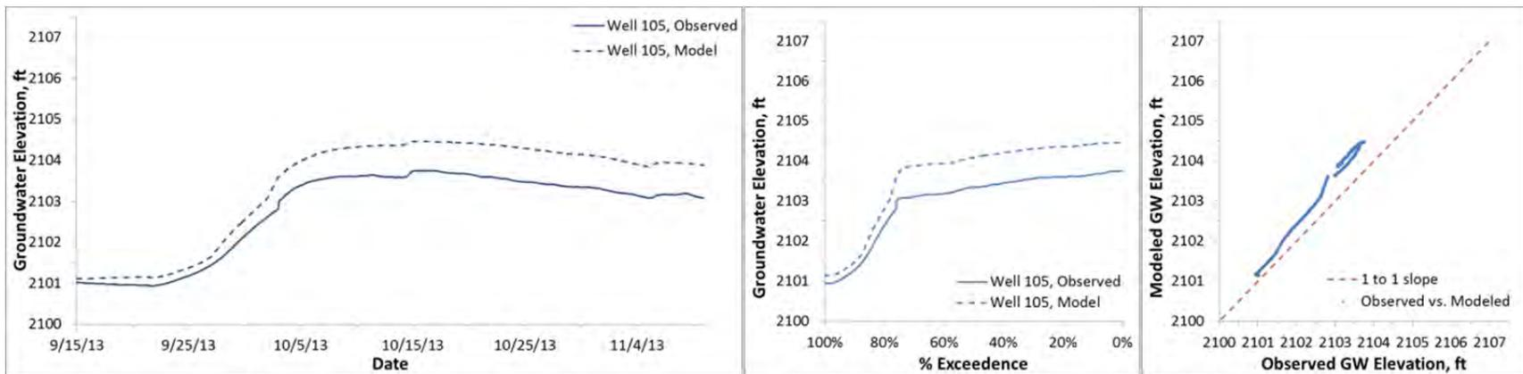
Figure D6. Modeled and observed heads, Fox well 105 (ground surface elevation 2107.7 ft)
