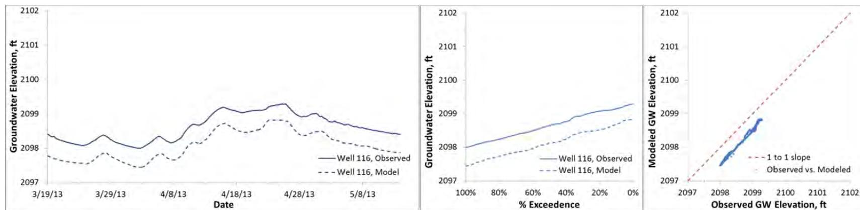
Figure C10. Modeled and observed heads, Fox well 116 (ground surface elevation 2105.0 ft)
