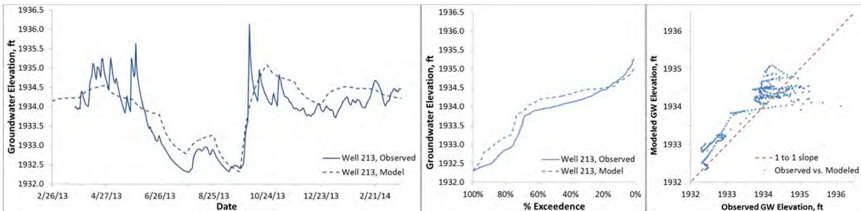
Figure B29. Modeled and observed heads 2013-2014, Binfield well 213 (ground surface elevation 1937.3 ft)
