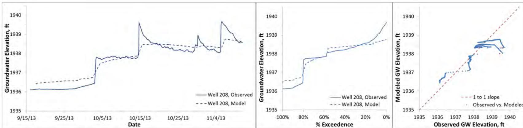
Figure D24. Modeled and observed heads, Binfield well 208 (ground surface elevation 1940.4 ft)
