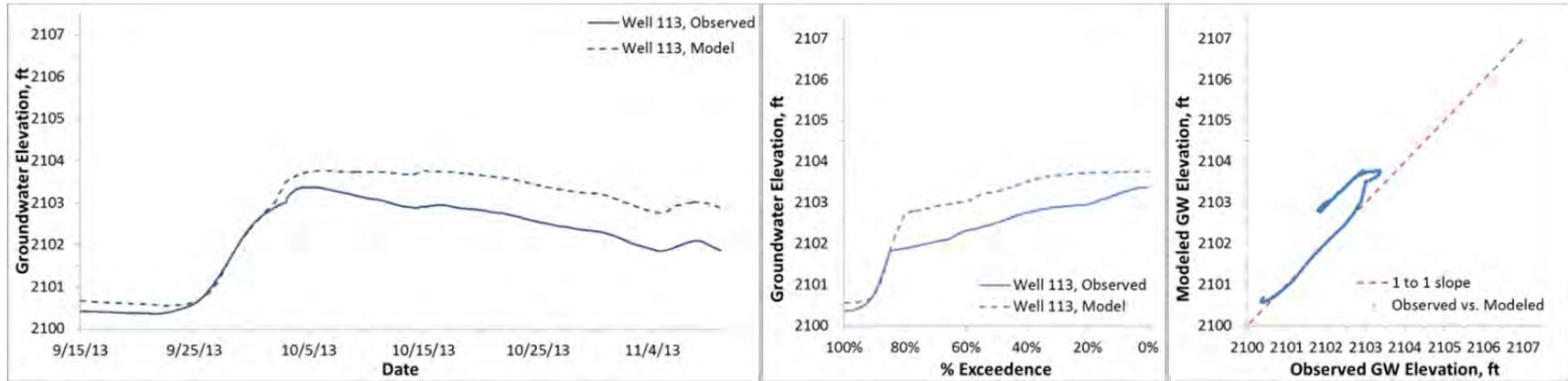
Figure D9. Modeled and observed heads, Fox well 113 (ground surface elevation 2107.6 ft)
