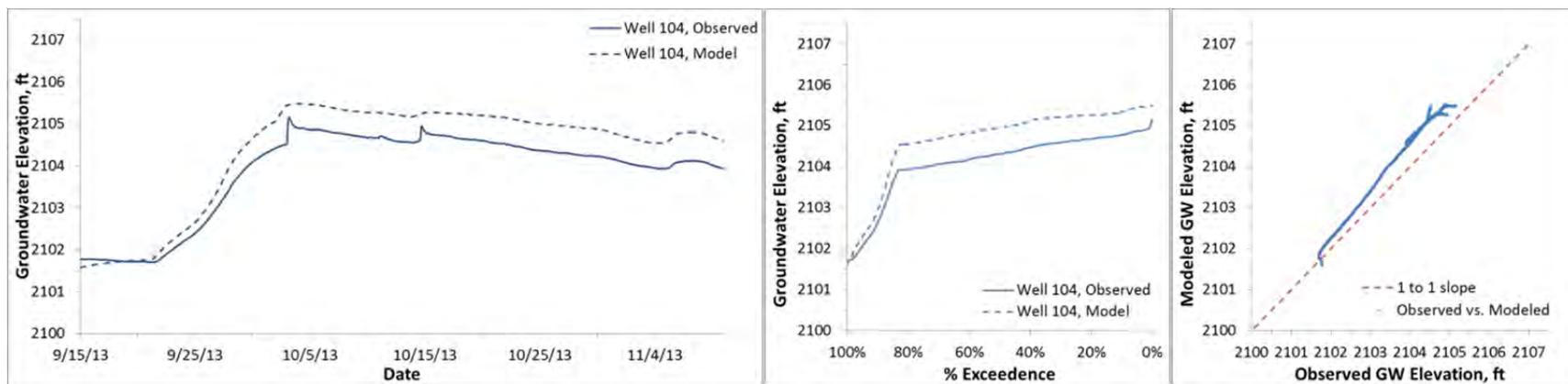
Figure D4. Modeled and observed heads, Fox well 104 (ground surface elevation 2107.1 ft)
