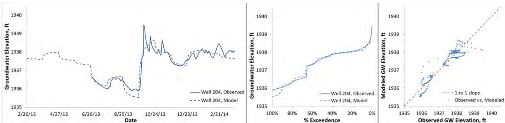
Figure B20. Modeled and observed heads 2013-2014, Binfield well 204 (ground surface elevation 1941.4 ft)
