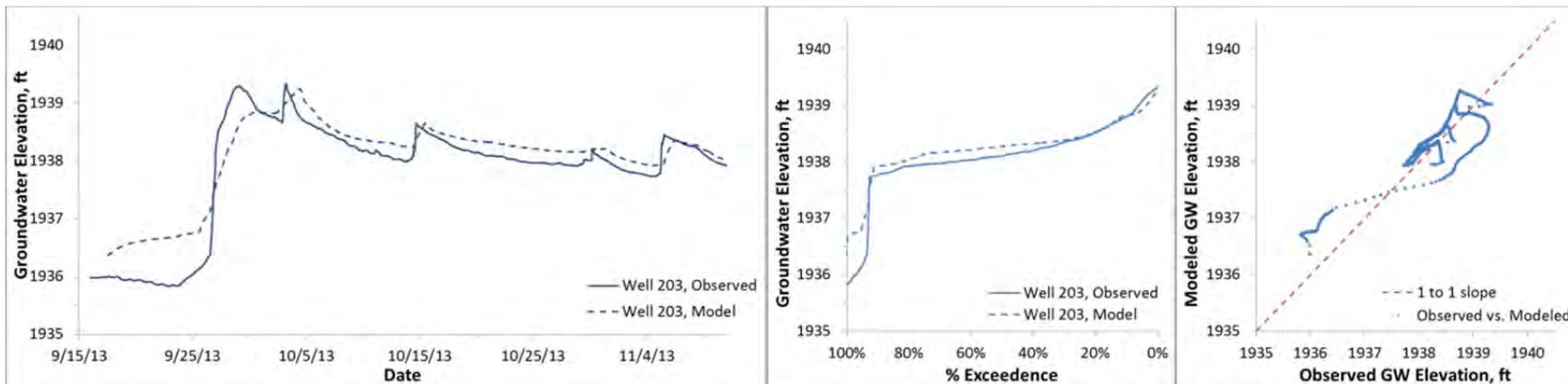
Figure D19. Modeled and observed heads, Binfield well 203 (ground surface elevation 1939.4 ft)
