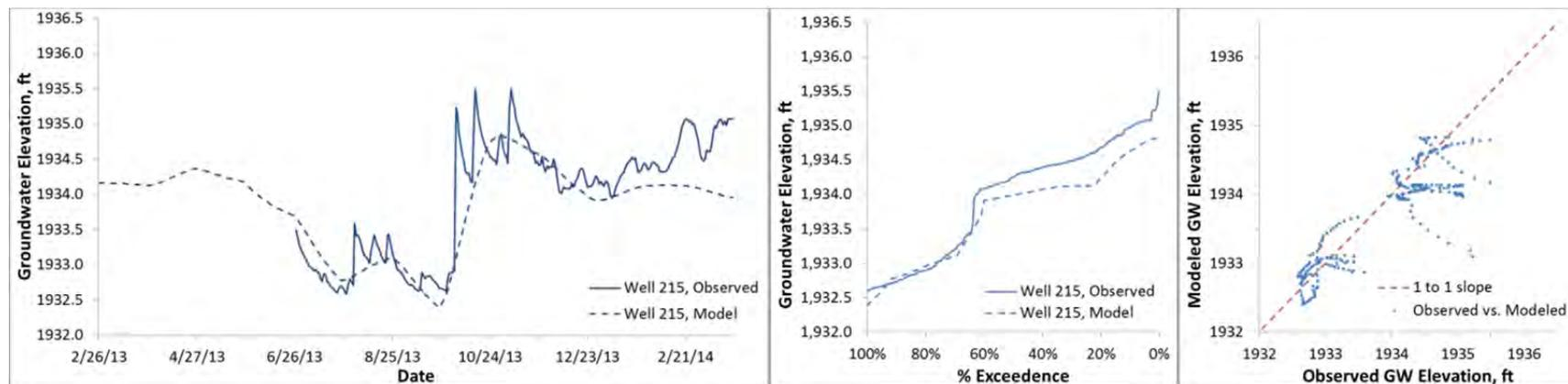
Figure B31. Modeled and observed heads 2013-2014, Binfield well 215 (ground surface elevation 1936.4 ft)
