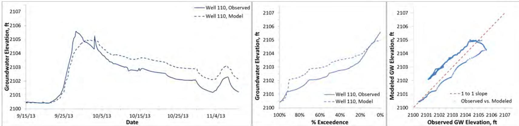
Figure D12. Modeled and observed heads, Fox well 110 (ground surface elevation 2108.9 ft)
