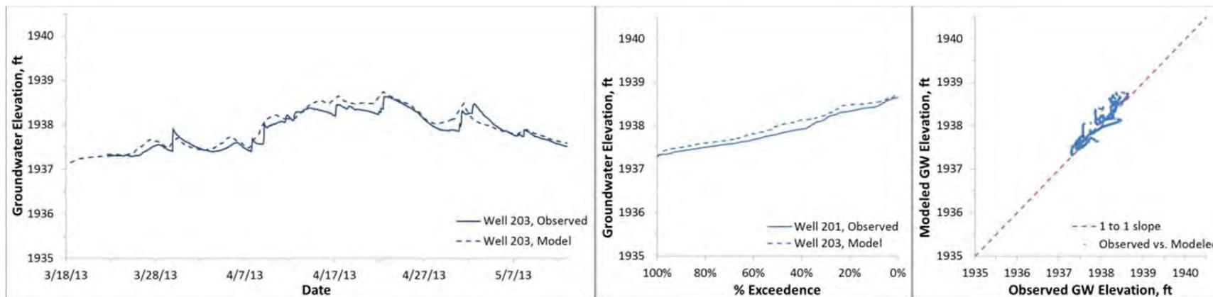
Figure C12. Modeled and observed heads, Binfield well 203 (ground surface elevation 1939.4 ft)
