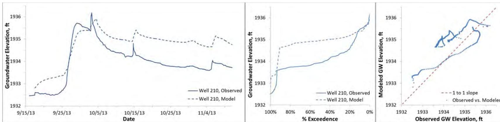
Figure D26. Modeled and observed heads, Binfield well 210 (ground surface elevation 1937.3 ft)
