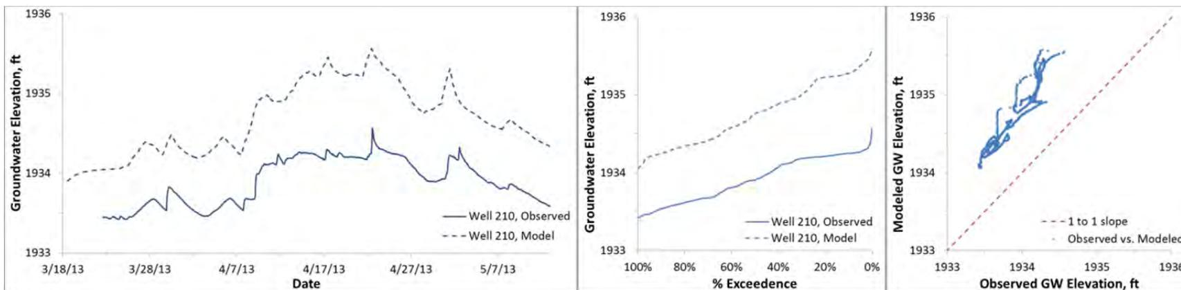
**Figure C15.** Modeled and observed heads, Binfield well 210 (ground surface elevation 1937.3 ft)
