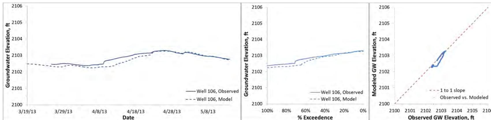
Figure C4. Modeled and observed heads, Fox well 106 (ground surface elevation 2107.7 ft)
