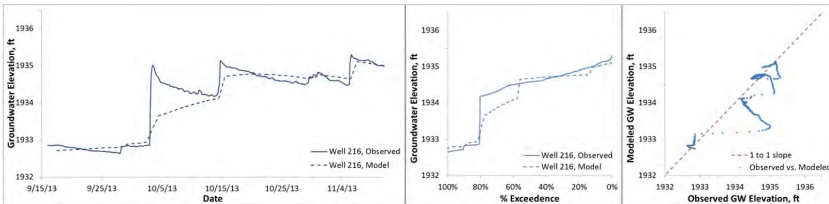
Figure D32. Modeled and observed heads, Binfield well 216 (ground surface elevation 1936.3 ft)
