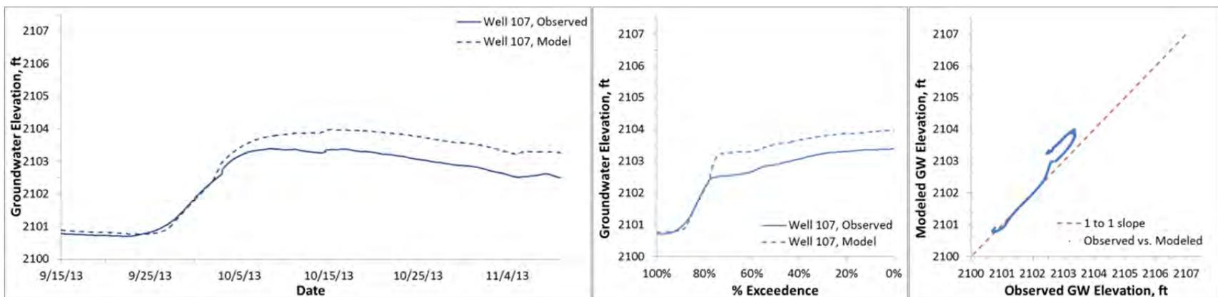
Figure D8. Modeled and observed heads, Fox well 107 (ground surface elevation 2107.7 ft)
