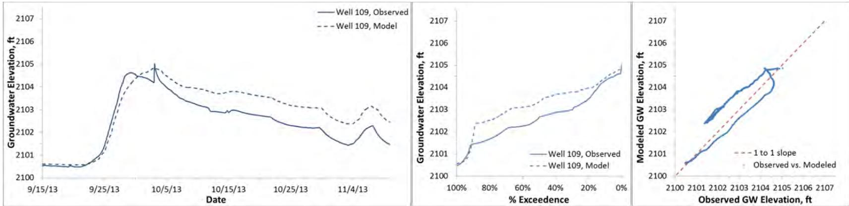
Figure D11. Modeled and observed heads, Fox well 109 (ground surface elevation 2108.1 ft)
