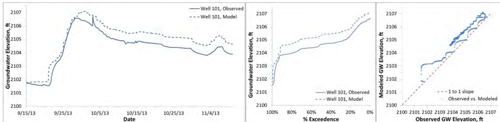
**Figure D1.** Modeled and observed heads, Fox well 101 (ground surface elevation 2110.1 ft)
