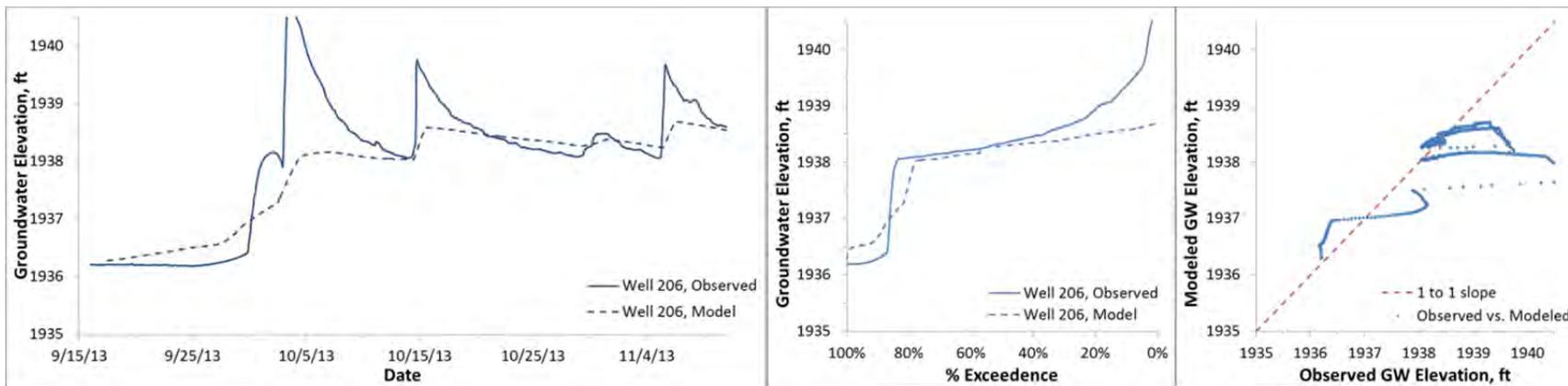
**Figure D22.** Modeled and observed heads, Binfield well 206 (ground surface elevation 1940.8 ft)
