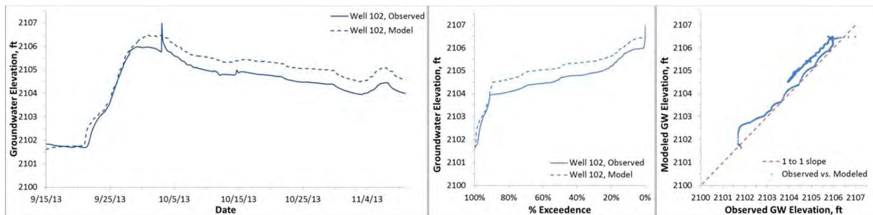
**Figure D2.** Modeled and observed heads, Fox well 102 (ground surface elevation 2109.6 ft)
