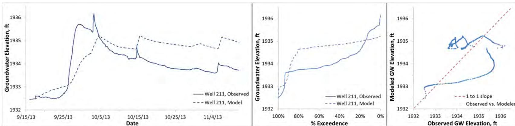
Figure D27. Modeled and observed heads, Binfield well 211 (ground surface elevation 1937.8 ft)
