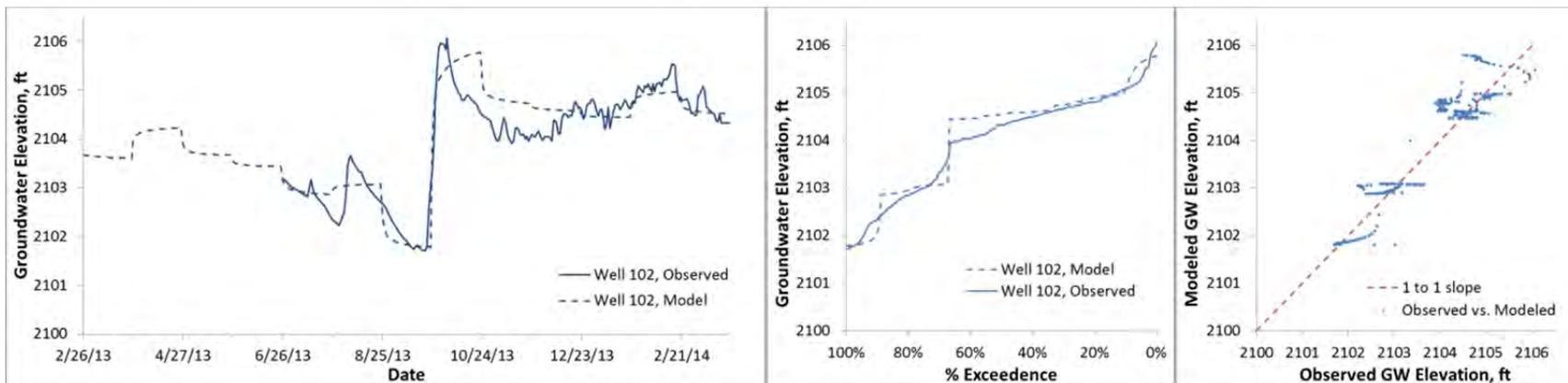
759 **Figure B2.** Modeled and observed heads 2013-2014, Fox well 102 (ground surface elevation 2109.6 ft)
