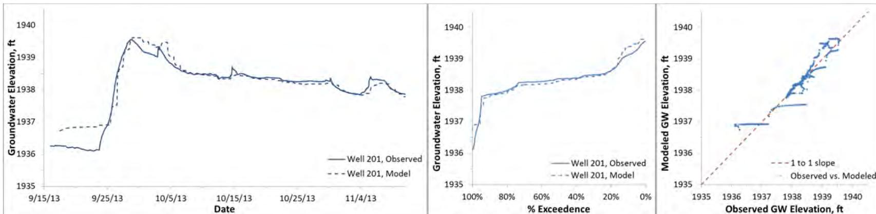
Figure D17. Modeled and observed heads, Binfield well 201 (ground surface elevation 1939.2 ft)
