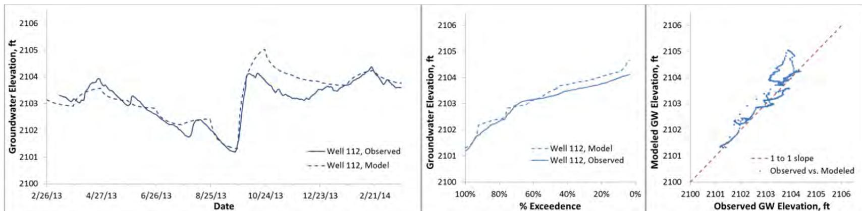
**Figure B5.** Modeled and observed heads 2013-2014, Fox well 112 (ground surface elevation 2107.4 ft)
