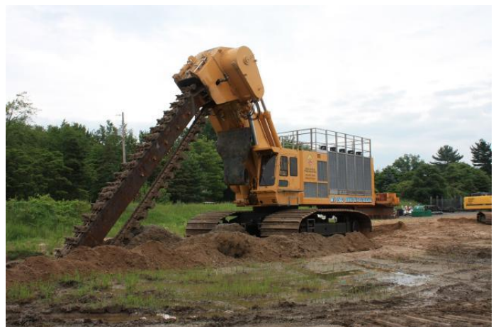
Figure 4 - Alternate slurry trenching equipment
