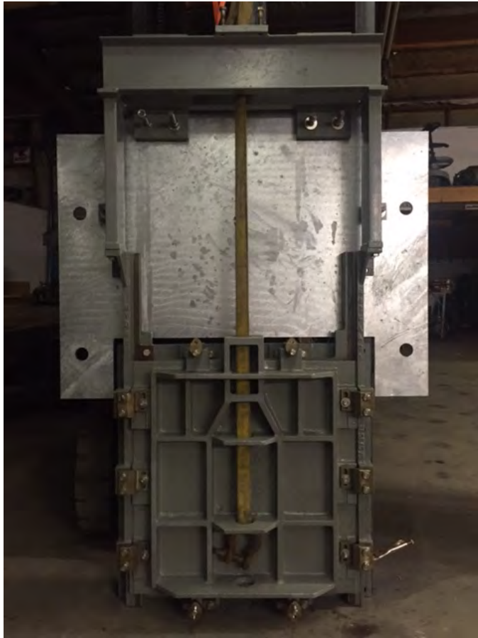
Photograph 14: April 27, 2016. 30-inch Slide Gate (Second installation) and Stiffener Plate.
