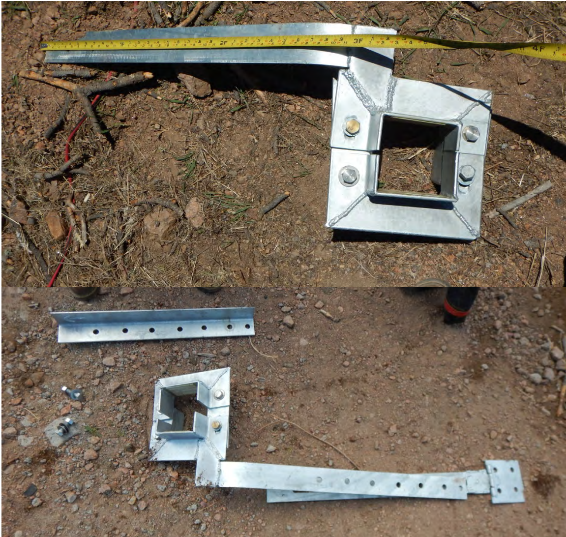
Photograph 18: May 12, 2016. Hydraulic cylinder support bracket (30-inch slide gate).
