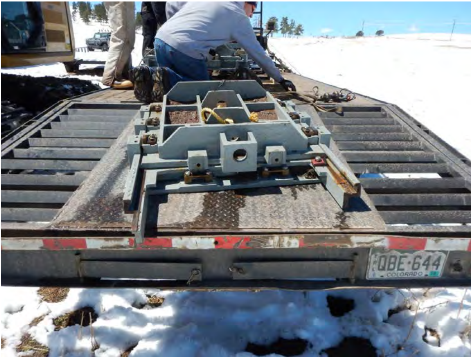
Photograph 13: May 2, 2016. Remains of the 30-inch slide gate (first installation) removed from the Reservoir.
