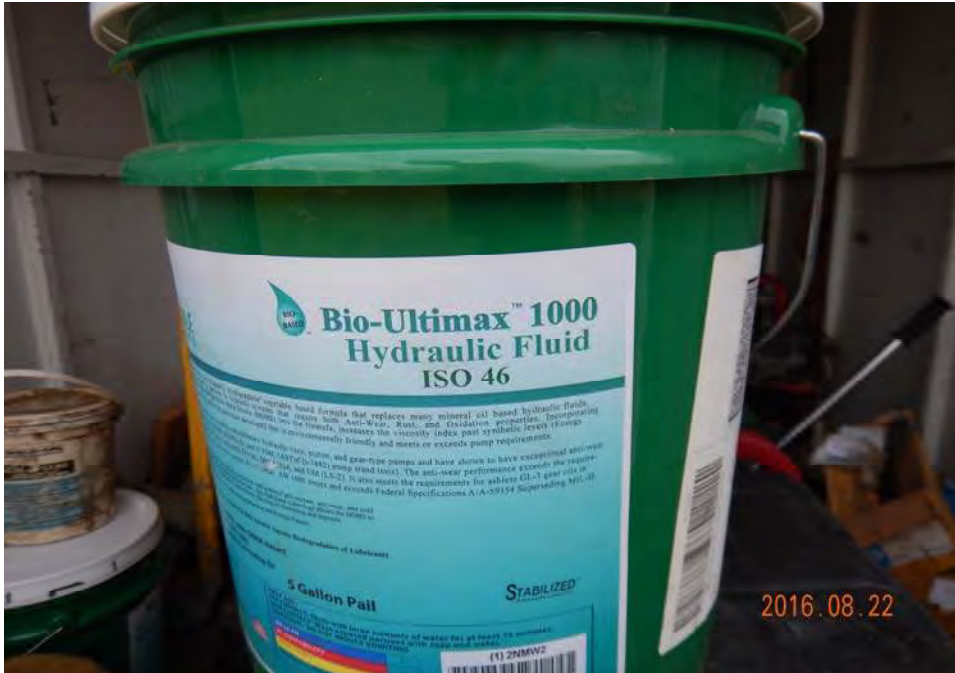
Photograph 43: Hydraulic fluid used for the gate.
