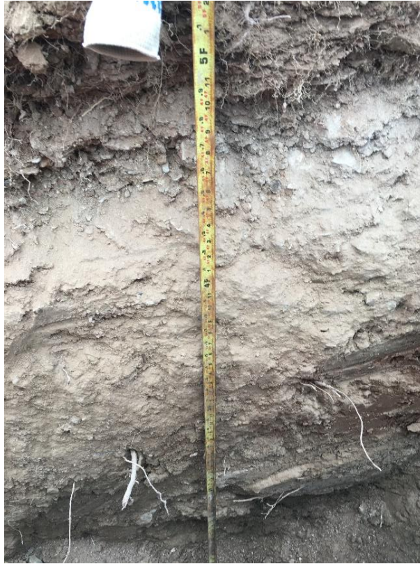
TP- 1: Test pit wall with clayey fill soils overlying shale bedrock.
