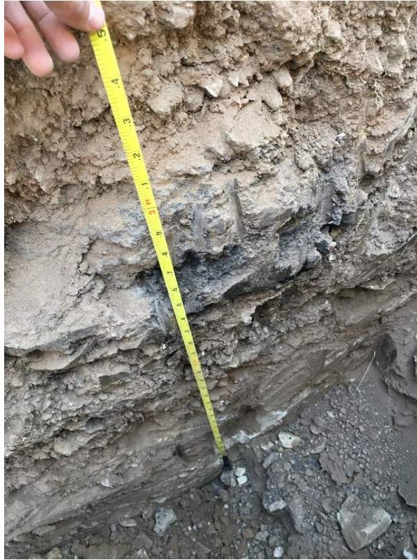
TP- 2: Test pit wall with clayey fill soils overlying shale bedrock.
