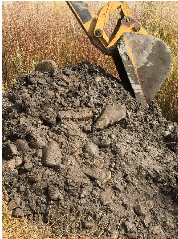
TP- 7: Excavated pile of saturated alluvial soils.
