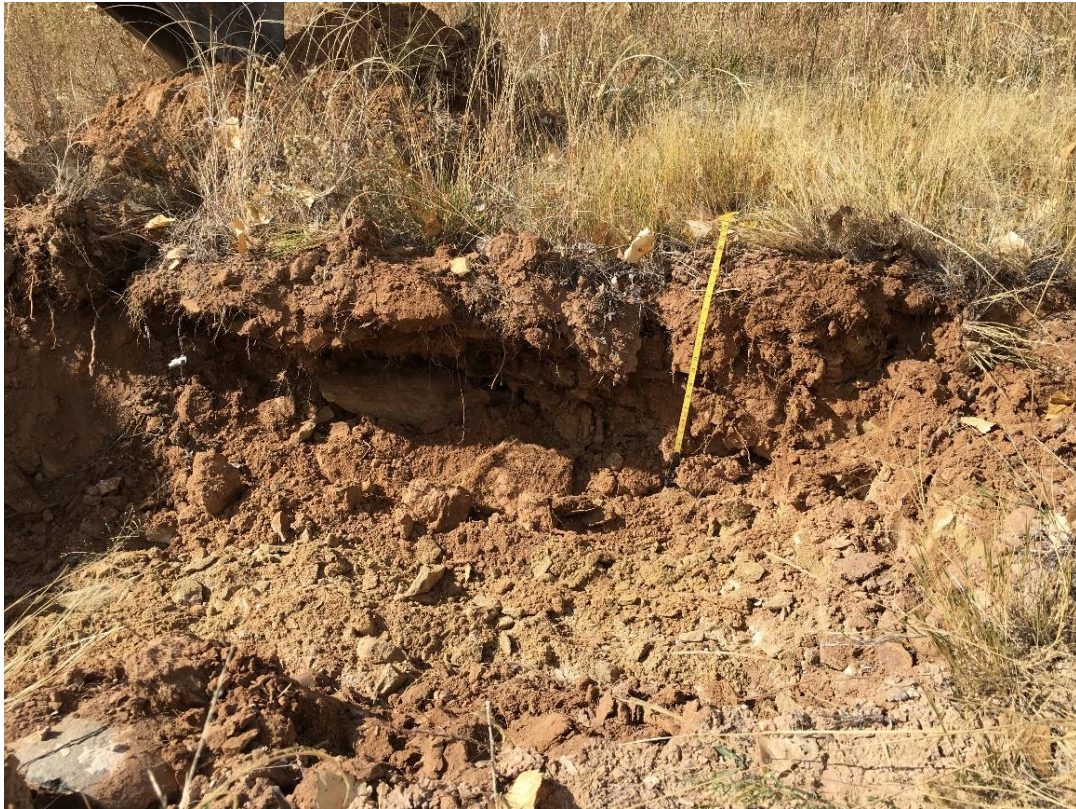
TP- 5: Shallow test pit showing very hard pale yellow sandstone bed.
