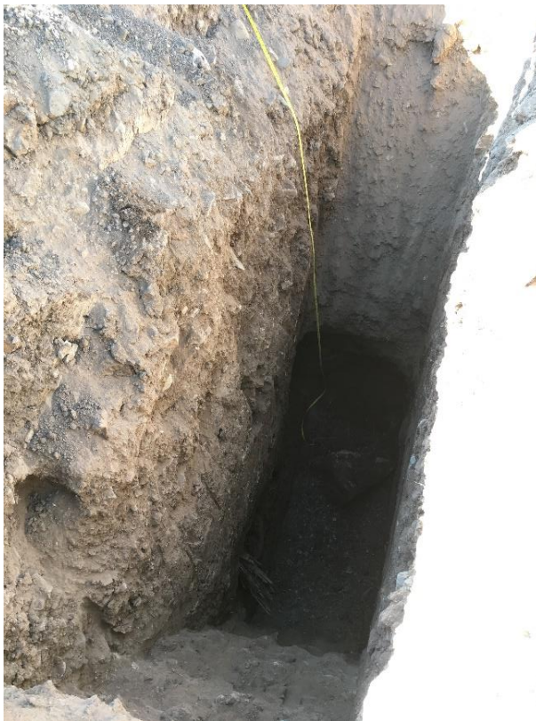
TP- 4: Test pit with fill soils overlying shale bedrock.
