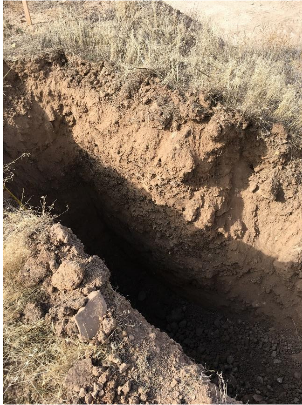
TP- 3: Test pit with clayey sand and gravel fill.
