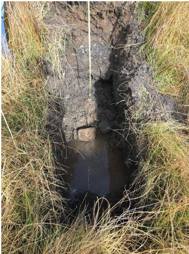
TP- 8: Floodplain deposits overlying saturated alluvial sand and gravel with large cobbles.
