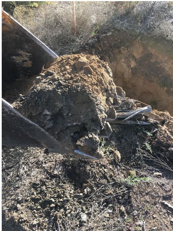
TP- 2: Fill soils and weathered shale bedrock excavated from test pit.
