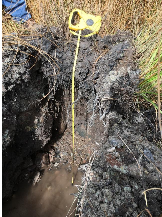
TP- 7: Floodplain deposits overlying saturated alluvial sand and gravel with large cobbles.
