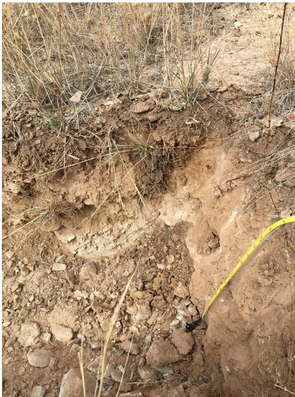
TP- 6: Shallow test pit showing hard pale yellow sandstone bed on bottom.
