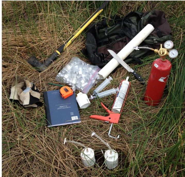
Figure 2: Equipment to test microbial denitrification, two installed incubation chambers located lower enter.
