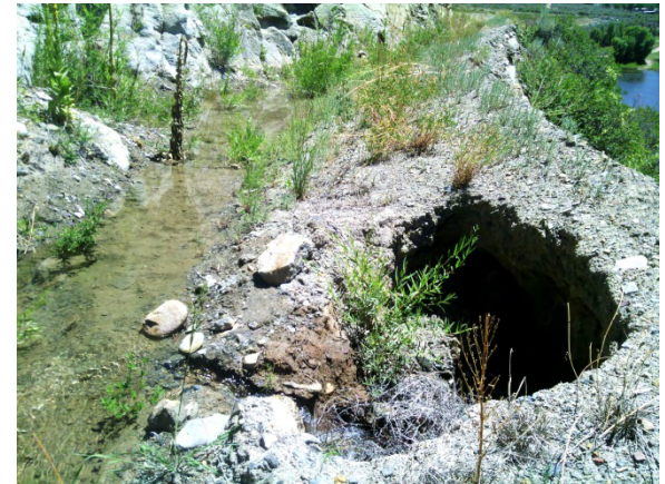
Photo 6: Sinkhole observed near ditch.
