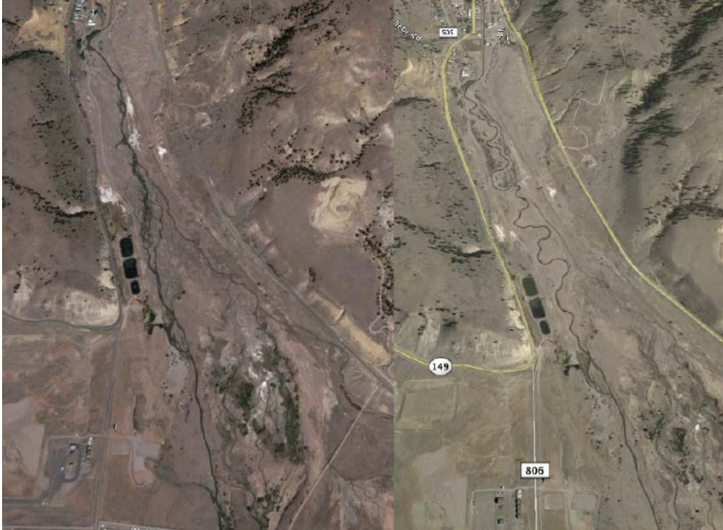
Figure 1: Photograph depicting the change in the Lower Willow Creek channel as part of Phase I. The photo on the left is the condition of the channel from 1939 to 2012. The photo on the right is the channel after Phase II was completed (photos courtesy of Google Earth).
