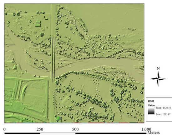
Figure 6a-d: Different Surfaces Generated from LiDAR Datasets.
