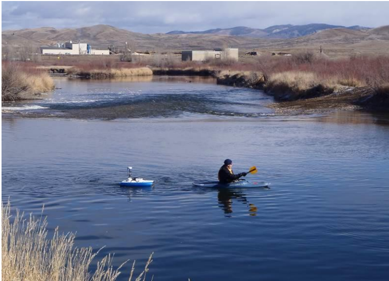
Figure 2 Acoustic Doppler Current Profiler (ADCP) Benthic Survey
