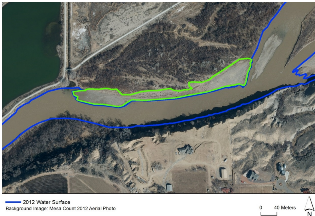
Figure 7 – Example comparison of water surface outline versus the non-vegetated active channel. The polygon outlined in green would be considered active channel, but would not be included if just the water surface were outlined.
