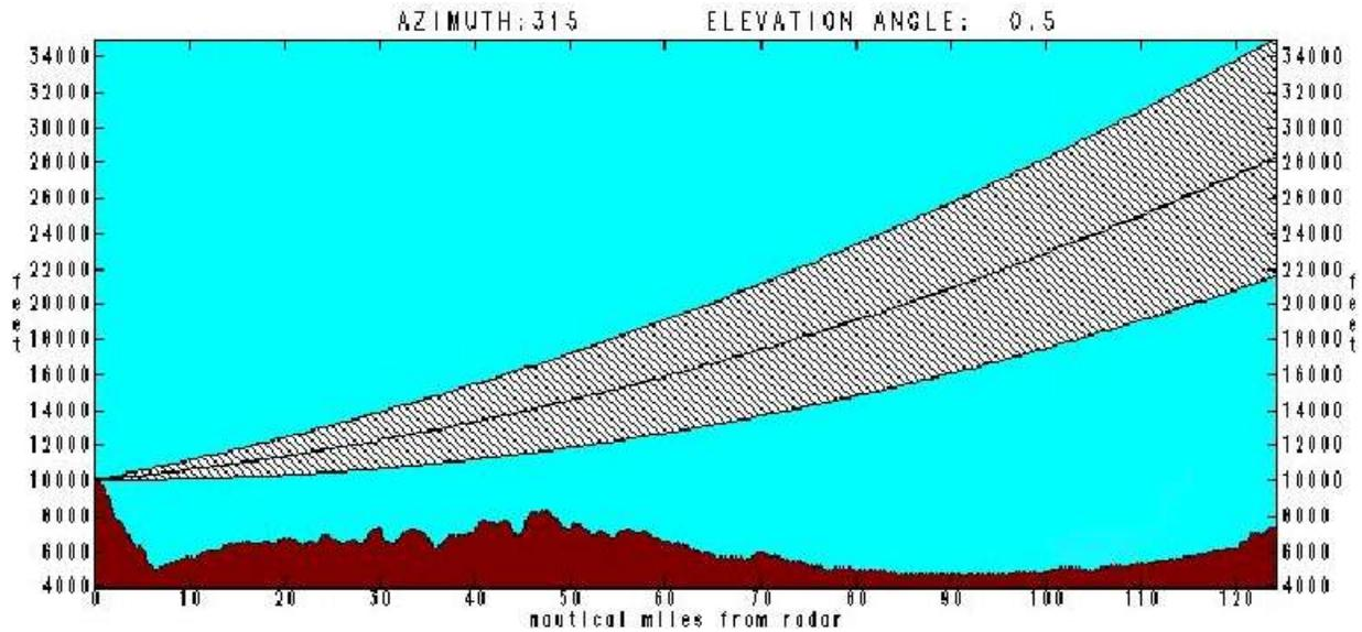
Figure 5. Schematic diagram of the 0.5 deg radar beam over complex terrain.
