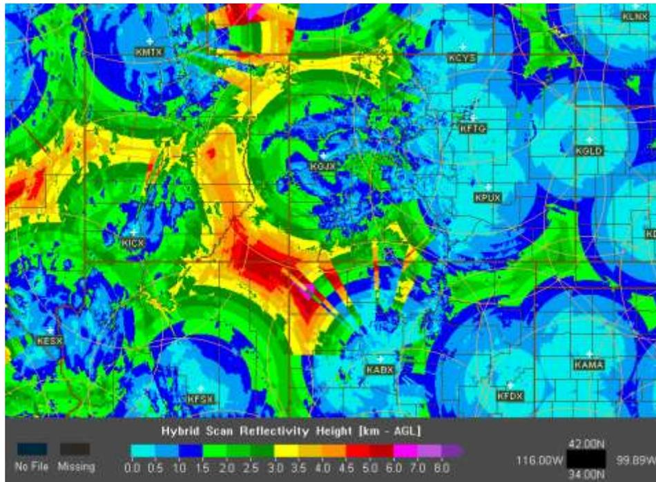
Figure 7. WSR-88D beam heights in km above ground level. Light blue indicates the best coverage.
