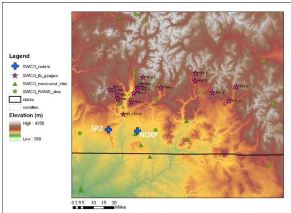
Figure 3. Locations of research tipping bucket rain gauges indicated by purple stars. Permanent gauges are indicated by green symbols. Mobile radar locations are indicated by blue + signs. Note that Ft. Lewis is in Durango. SR2 is on Bridge Timber Mountain and NOXP is at the Durango – La Plata County Airport. Terrain elevation is color coded with higher terrain in white.
