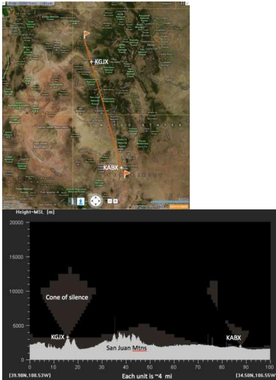
Figure 8. Top panel shows the location of the vertical cross section between KGJX and KABQ shown in lower panel. Grey shading above the white terrain indicates no coverage.
