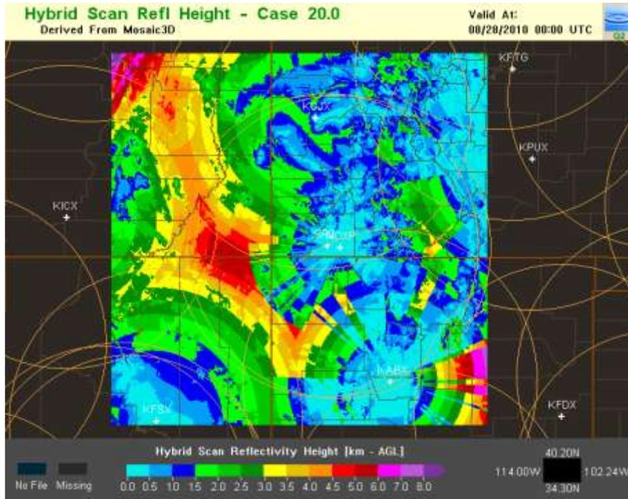
Figure 10. Radar beam heights in km above ground level as in figure 7 except with the NOXP coverage added. Light blue indicates the best coverage close to the ground.
