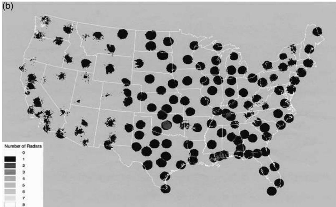
Figure 4. WSR-88D coverage below 1 km above ground level. From Maddox et al. 2002.
