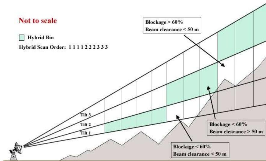
Figure 6. Schematic diagram showing how a hybrid scan is created from different elevation angles. Rules for deciding which bins to use are indicated.
