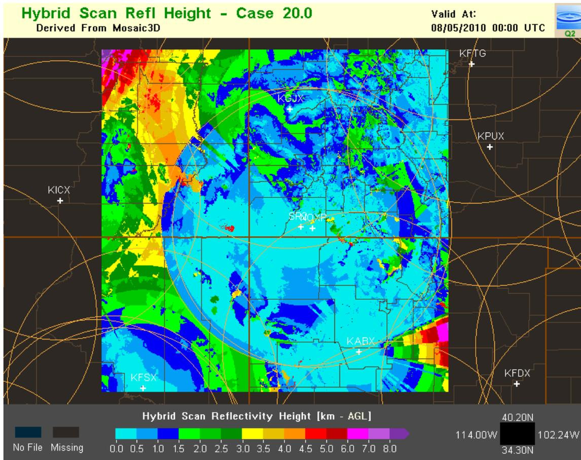
Figure 13. Radar beam heights in km above ground level as in figure 7 except with the SR2 coverage added. Light blue indicates the best coverage.
