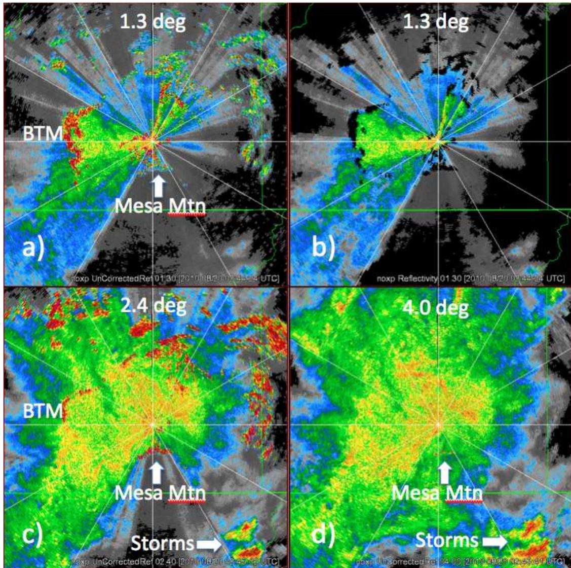
Figure 11. Reflectivity images from the NOXP at a) 1.3 deg, b) 1.3 deg with clutter filter applied, c) 2.4 deg, and d) 4.0 deg. Blue indicates light rain, yellow moderate rain, and red ground clutter except for actual storms at lower right.
