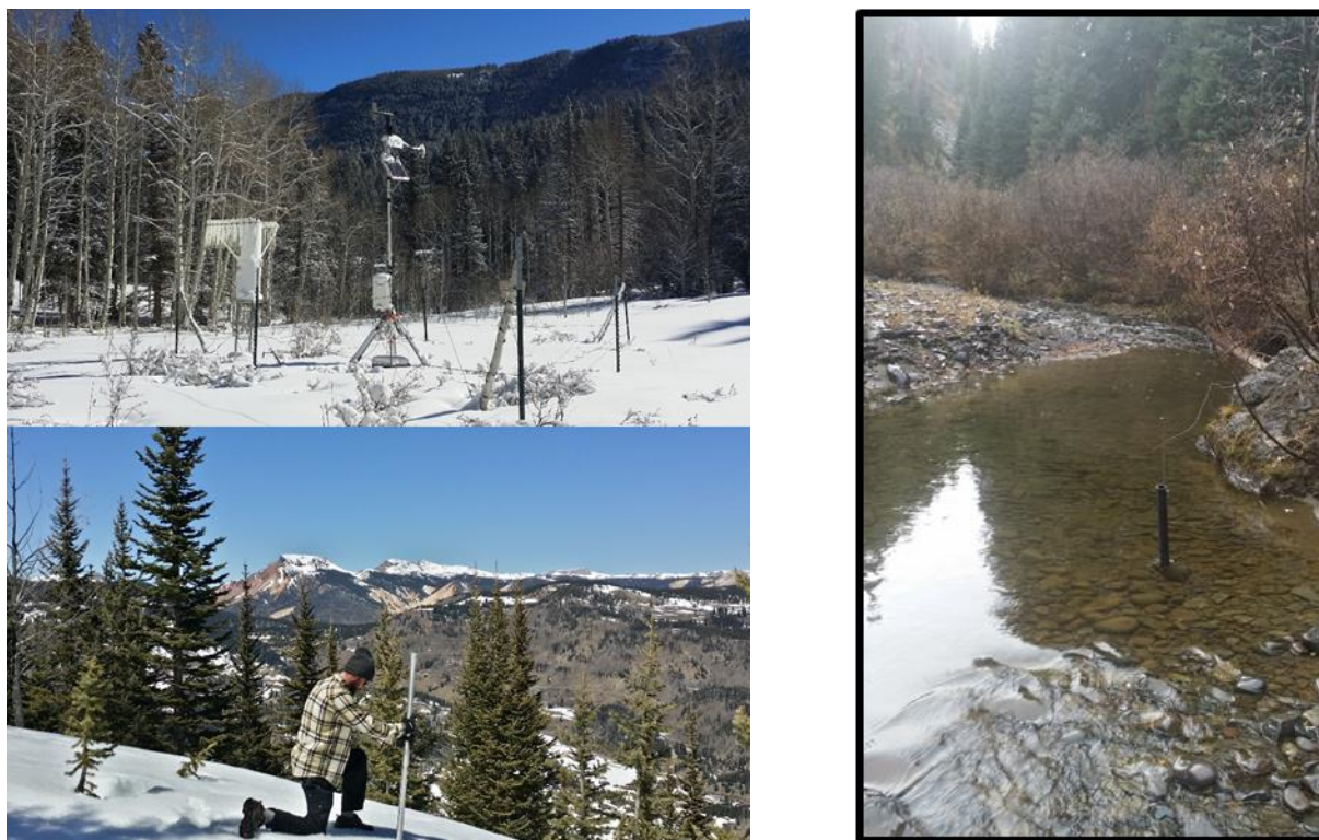
Figure 22. From top, left photo of SNO-LITE and right is river stage monitoring station. Bottom is a NCAR technician making manual snow density estimate
