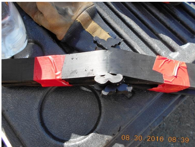
Bent Strap Test Coupon Showing Good Weld
