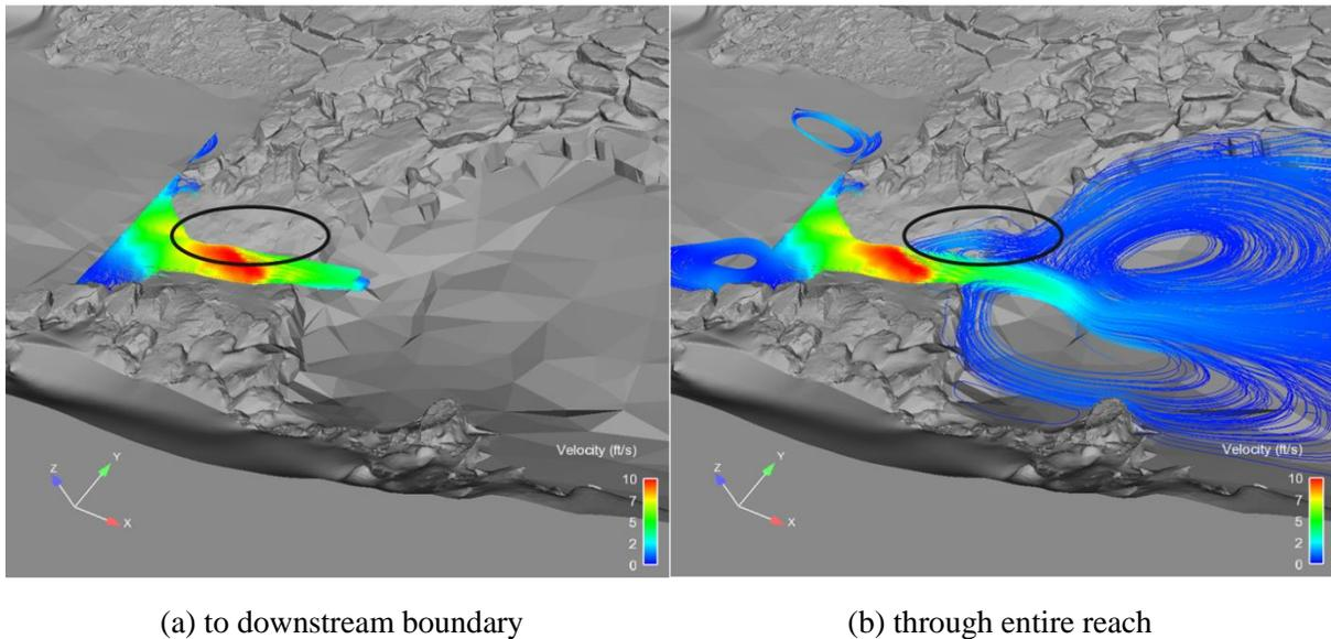
**Figure 3.4. (a) Particle traces released forward in time from an upstream cross section traveling to the downstream boundary, and (b) particle traces released forward from an upstream cross section traveling through the entire reach (Stephens, 2014). A reference recirculation zone is highlighted by a circle.**
