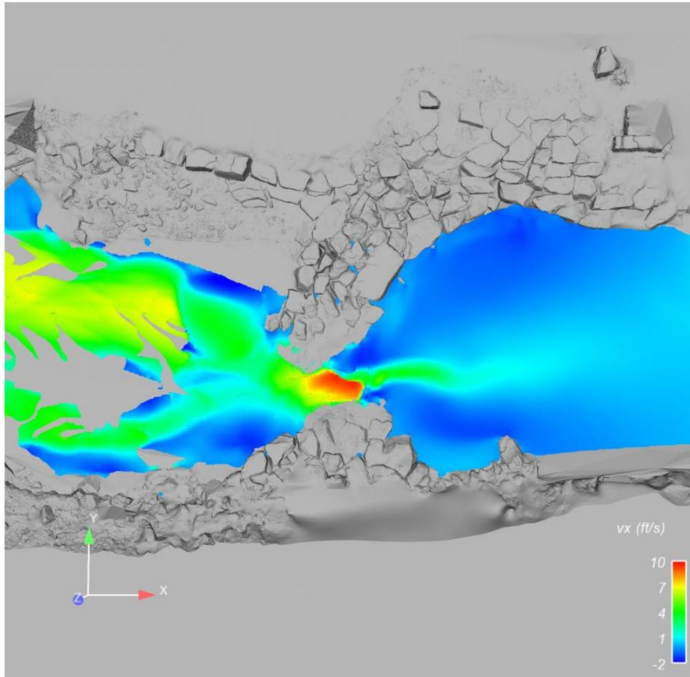
**Figure 3.6. Plan view of a WWP structure colored by velocity along the  $x$ -axis indicating flow moving upstream or downstream (Stephens, 2014).**
