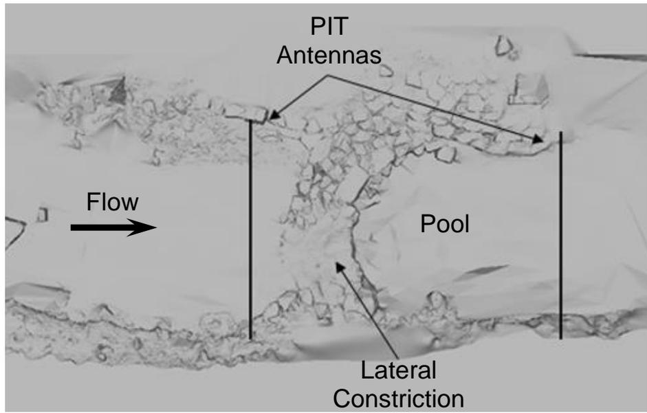
**Figure 3.1. Plan view of a WWP structure with PIT-antenna configuration (Stephens, 2014).**
