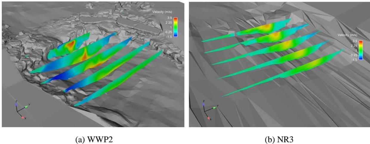
**Figure 1.3. Cross sections showing the downstream velocity component (m/s) in pools: (a) WWP2 and (b) NR3 at 4.25 cms (Kolden, 2013).**
