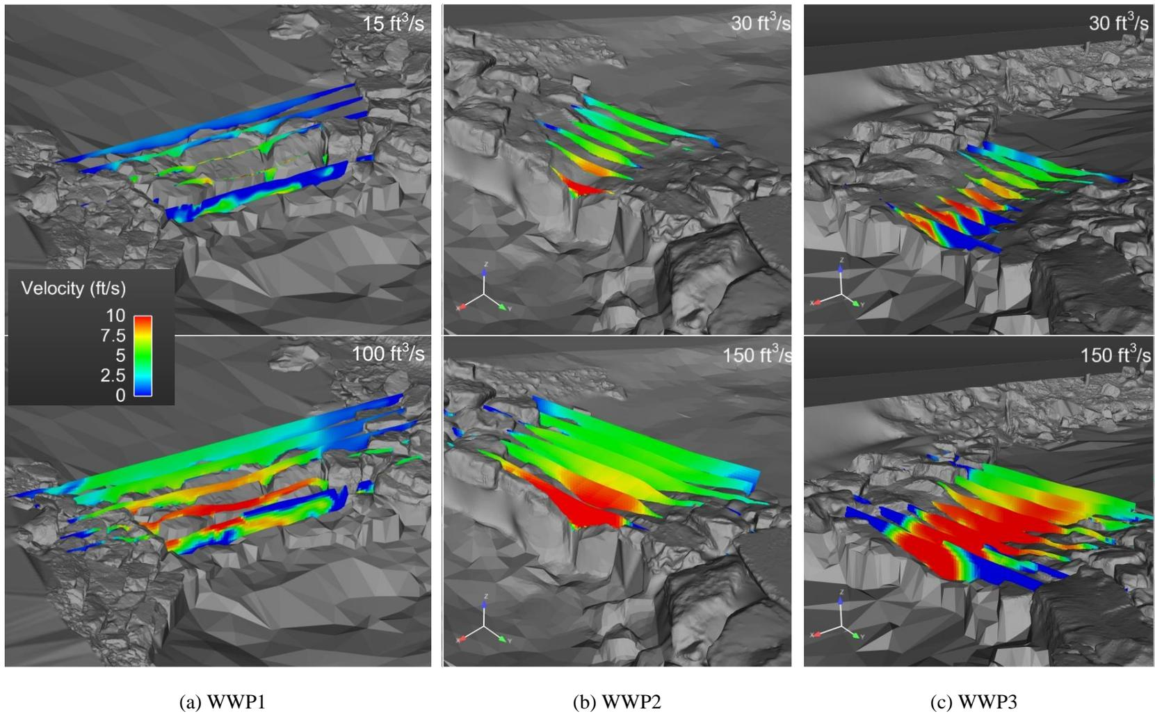
**Figure 2.12. Cross-sectional velocities for a low- and high-flow condition at: (a) WWP1; (b) WWP2; and (c) WWP3 (Fox, 2013).**
