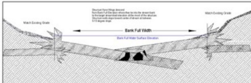
Cross Section B-B Log Rock & Roll Structure Profile Not To Scale
