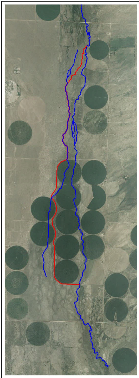
Figure 6: "Historic" (blue) and "relocated" (red) channels of San Luis Creek between Saguache County Road GG (north) and AA (south). Photo interpretation by Kelley Thompson, Colorado DWR, July, 2013.
