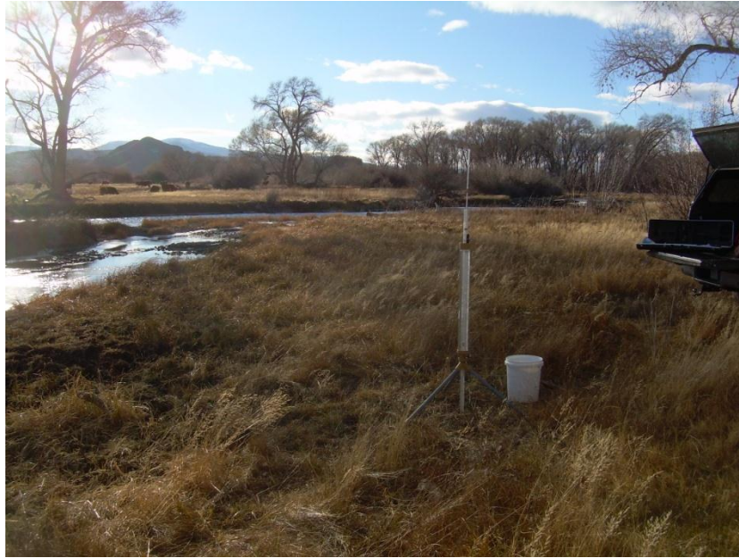
Figure 24: Field setup of Guelph constant-head permeameter. Near Kane-Callan headgate, looking upstream (west).
