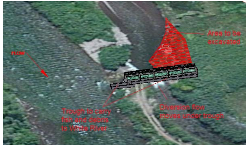
Figure 10 - Altered placement of the Coanda Screen
