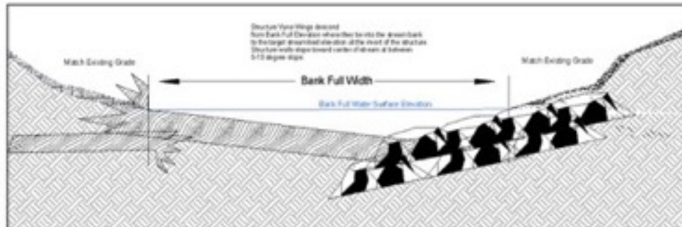
Cross Section B-B Log / Boulder J-Hook Vane Profile Not To Scale
