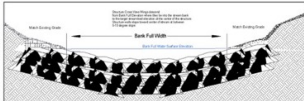
Cross Section B-B Boulder Cross Vane Profile
