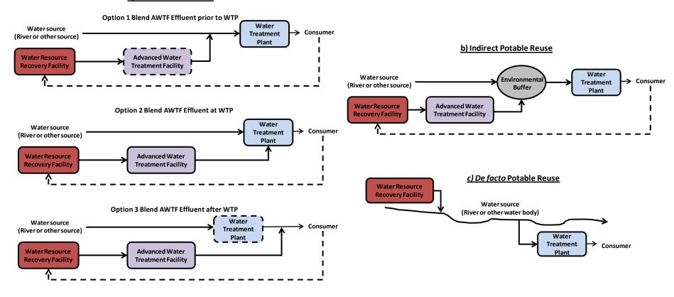
Figure 1-1. Simplified Comparison of (a) Direct, (b) Indirect and (c) De facto Potable Reuse.
