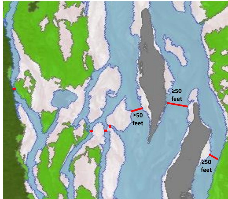
Figure 4. Channel width measured as the shortest distances across water from the edge of potentially suitable nesting areas to the bank lines on each side.
