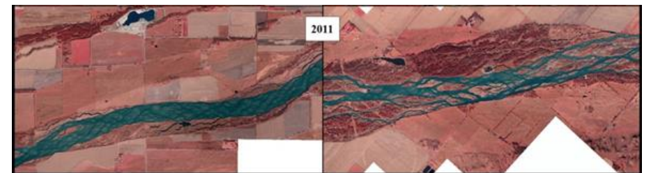
Figure 5. Two segment comparison of channel conditions following the drought of the 2000s. The mechanically managed Rowe Sanctuary segment (left) retained high habitat suitability. The unmanaged segment in the Grand Island to Chapman bridge segment (right) transitioned to an island braided planform during the drought. Mechanical clearing and leveling will be necessary to improve width suitability.
