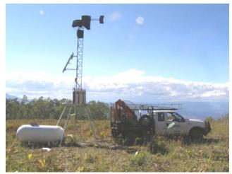
High elevation sites get silver in clouds, remote operated seeders put control to start and stop in the operator's hand, and data loggers and flow meters keep track of silver/hour totals for greater accountability and scientific analysis. Pictured is an Idaho Power technician installing a seeder above Collbran at 9300 feet MSL elevation. (*Joe Busto*)
