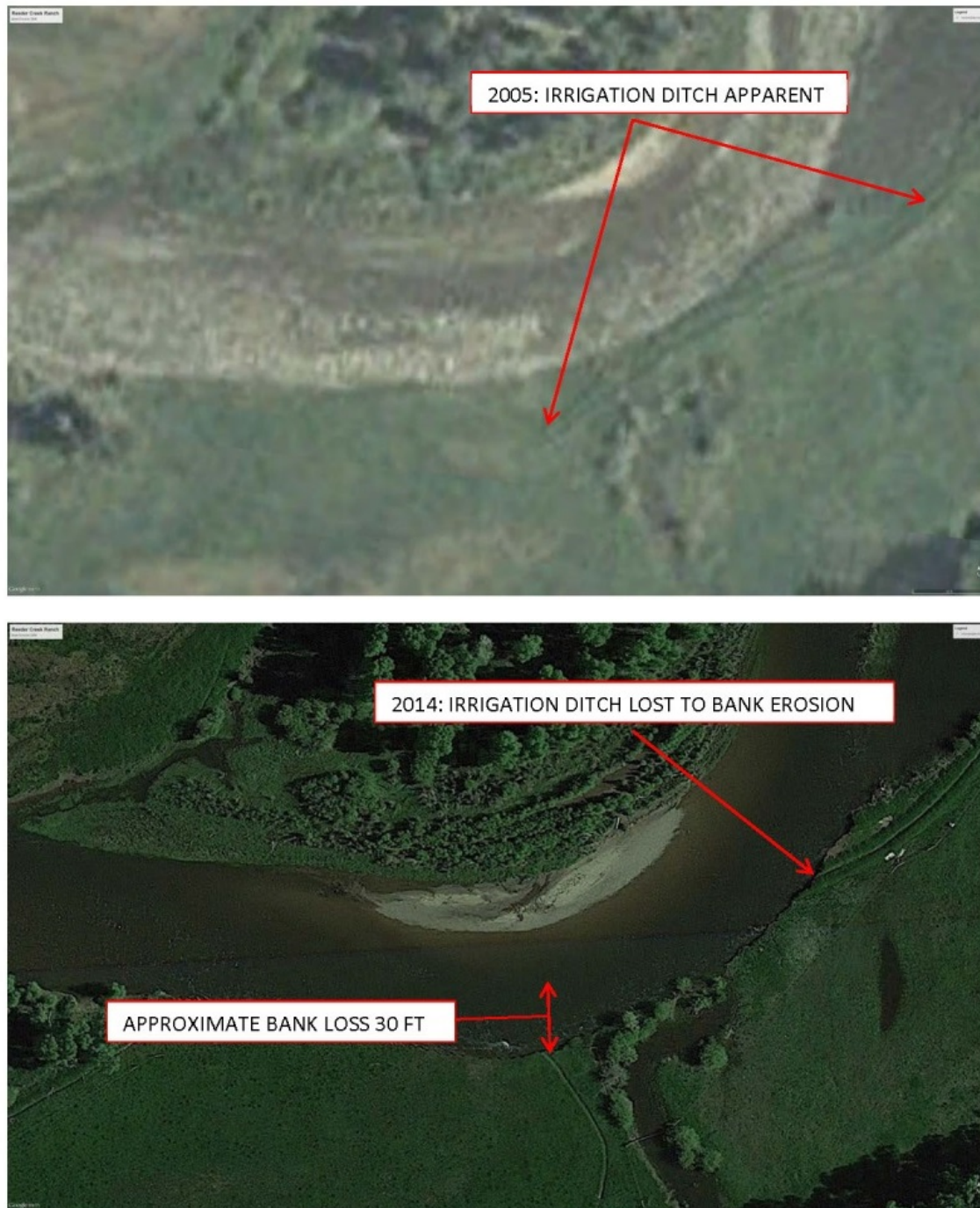
Figure 1-5. Sever Bank Erosion on Reeder Creek Ranch.
