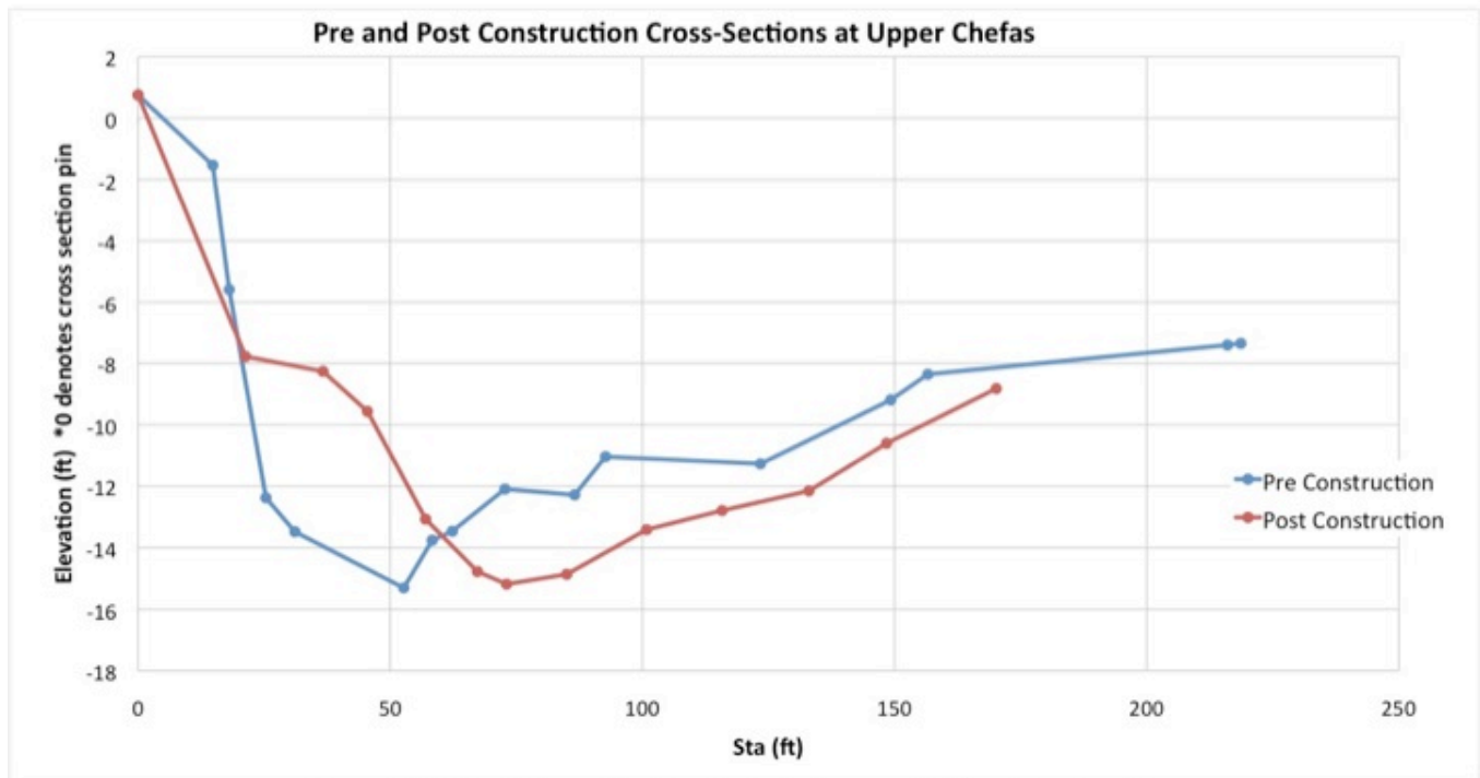
Figure 16. Site 2 Cross Section Data Before and After Construction.
