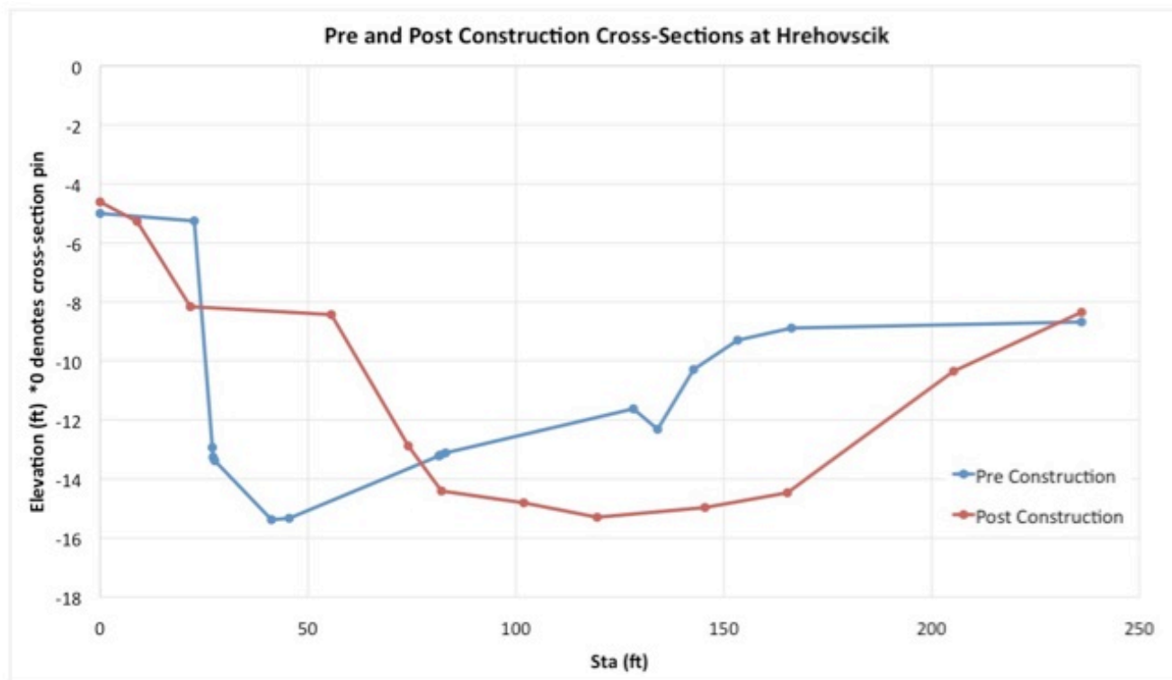
Figure 19. Site 3 Cross Section Data Before/After Construction.
