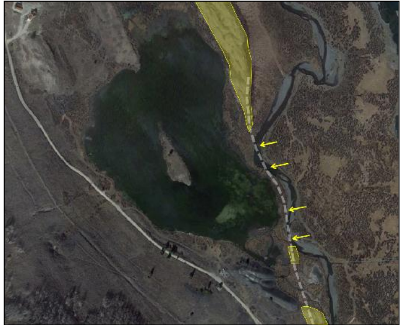
Figure 4: Peanut Lake showing the prominent bedrock ridge. Areas where the ridge is exposed are shaded in yellow. The yellow arrows show where the bedrock is exposed in the banks and bed of the river. The river has crossed the ridge at these two locations and is now on the same side as Peanut Lake.
