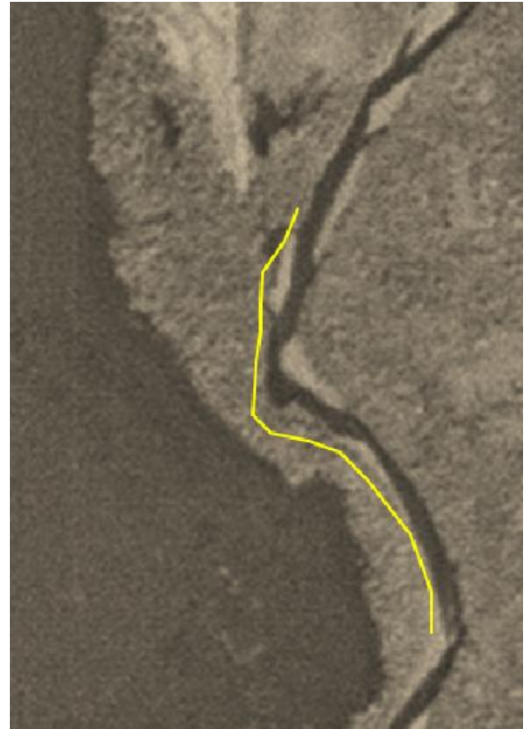
Figure 8: 1958 aerial showing the relatively similar alignment of the Slate River relative to Peanut Lake. The yellow line is an overlay of the right bank position in 2012 showing that the river has migrated 30-40 feet closer to the lake in 54 years.
