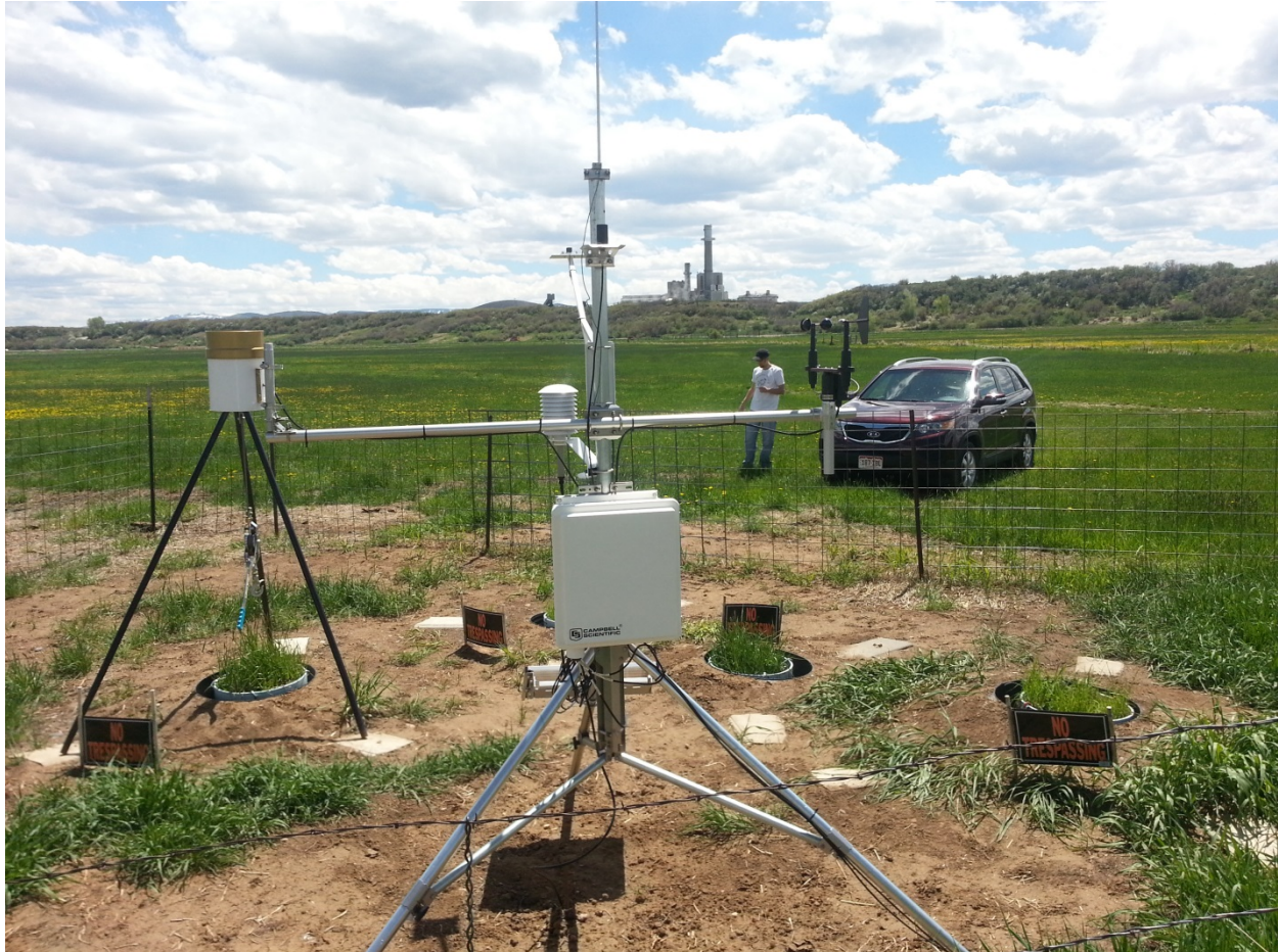
Figure 3: Site photo (looking South) with the lysimeter plots behind the station. Note the established grass within the lysimeter plots.
