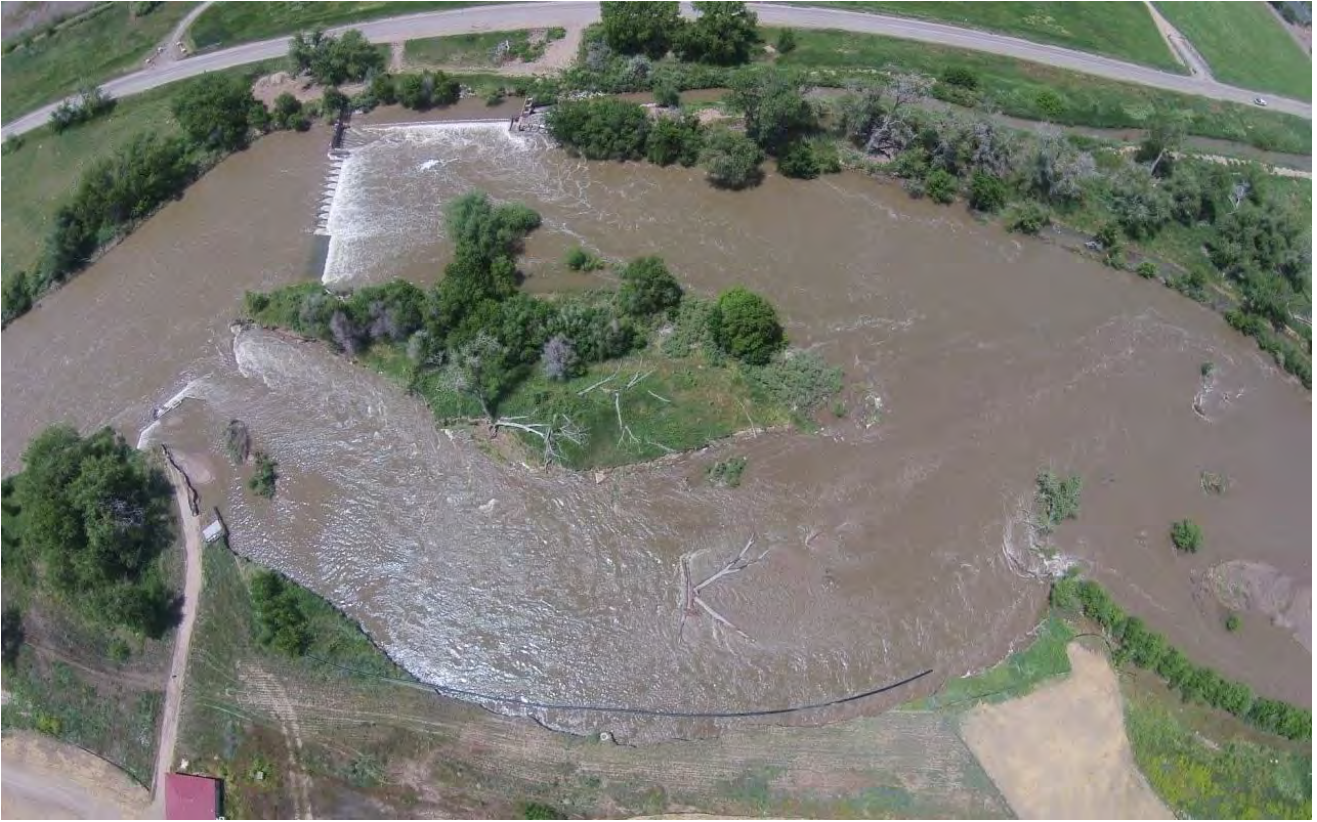
Photo 1: Aerial photo of breach site taken from east bank of the South Platte River looking west. Photo taken in early June 2015 (Photo provided by COA) shortly after the initial breach and while water flows were still high. BDC diversion structure is visible on the far bank. In foreground, the black pipe is a temporary surface pipe owned by COB. On left side of photo, the COB headgate and wing walls are visible at end of washed out road.
