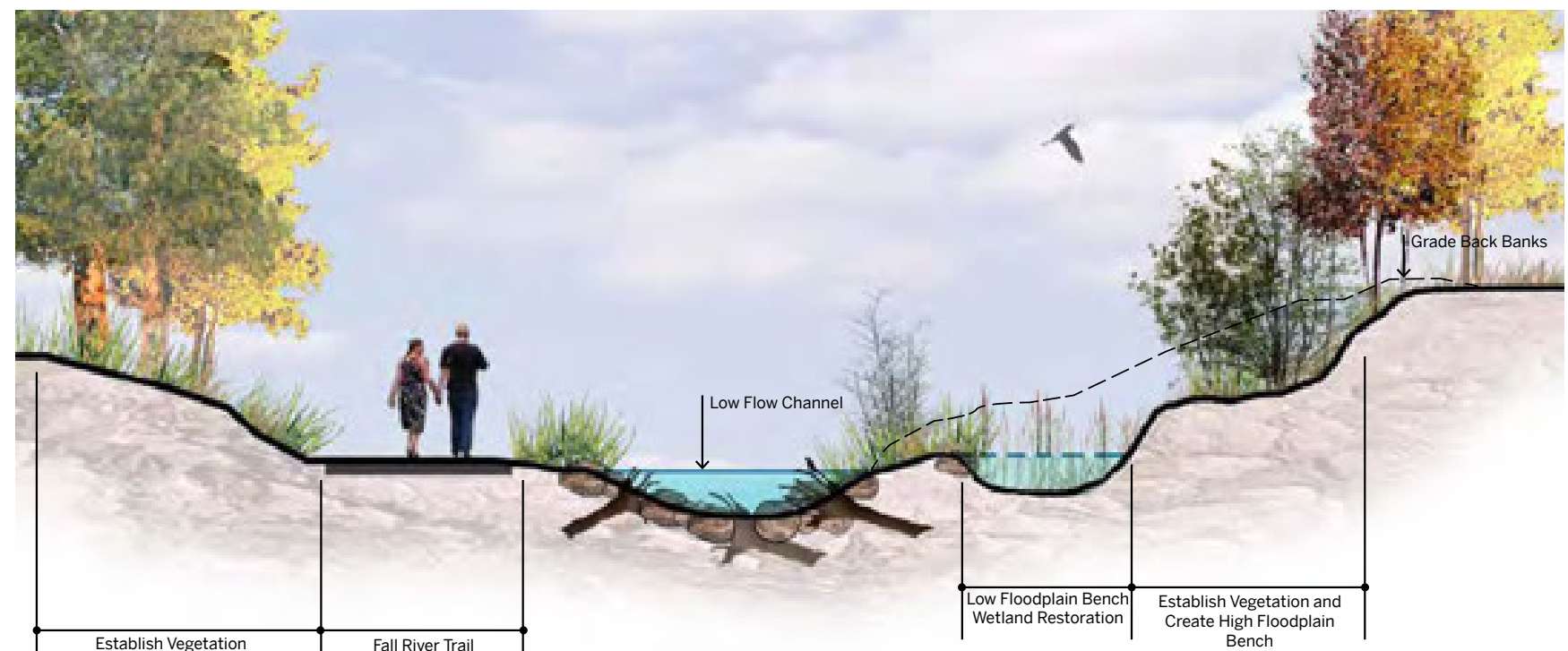
Figure 1. Compound channel for connected and variable floodplains. Compound or nested channels with floodplain benches below, at, and above the top of bank reduce flood surface elevations, maintain sediment transport while also providing refuge for fish and niches for diverse riparian plant communities.
