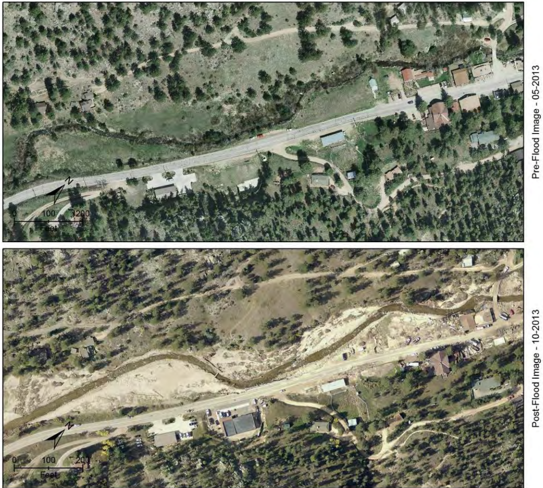
Figure 3.11. Section of West Creek that experienced degradation and aggradation, AHIP = 5.
