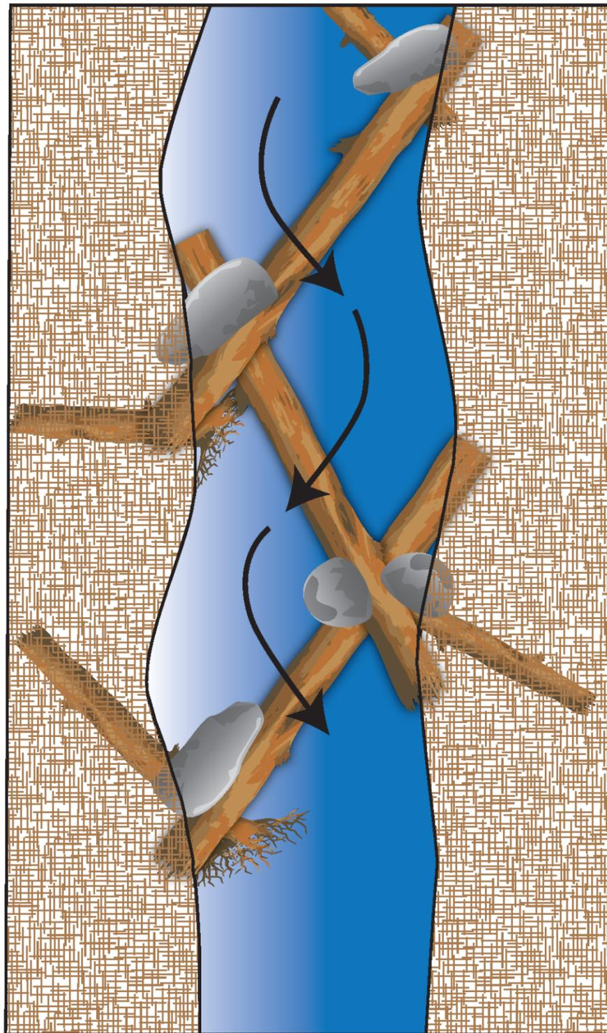
Figure 4-4. Log Roller Design in Plan View
