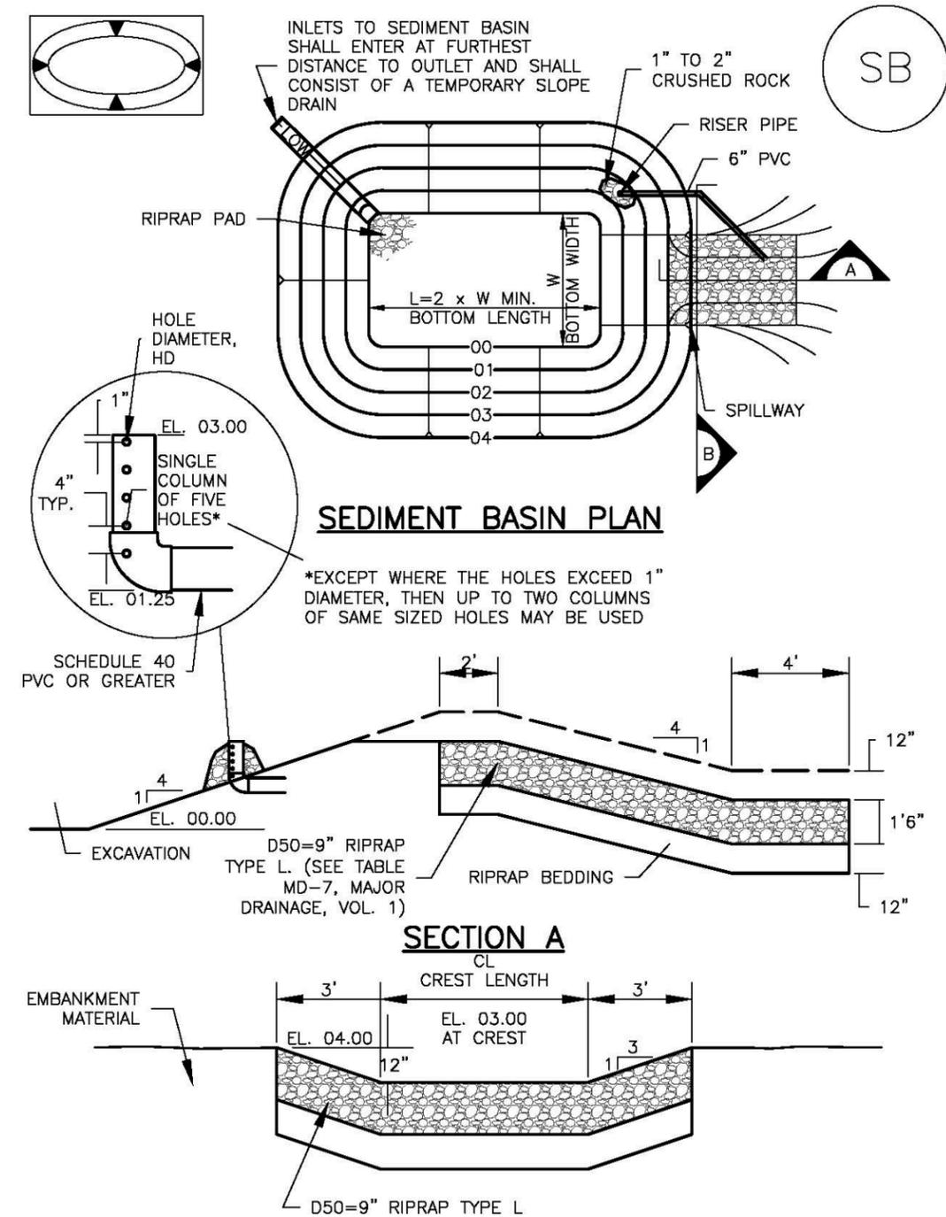
Figure 4-12. Sediment Basin Detail (from UDFCD Criteria Manual Vol. 3)
