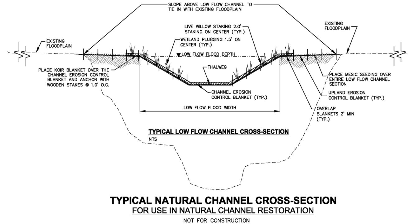
Figure 4-1. Natural Channel Section
