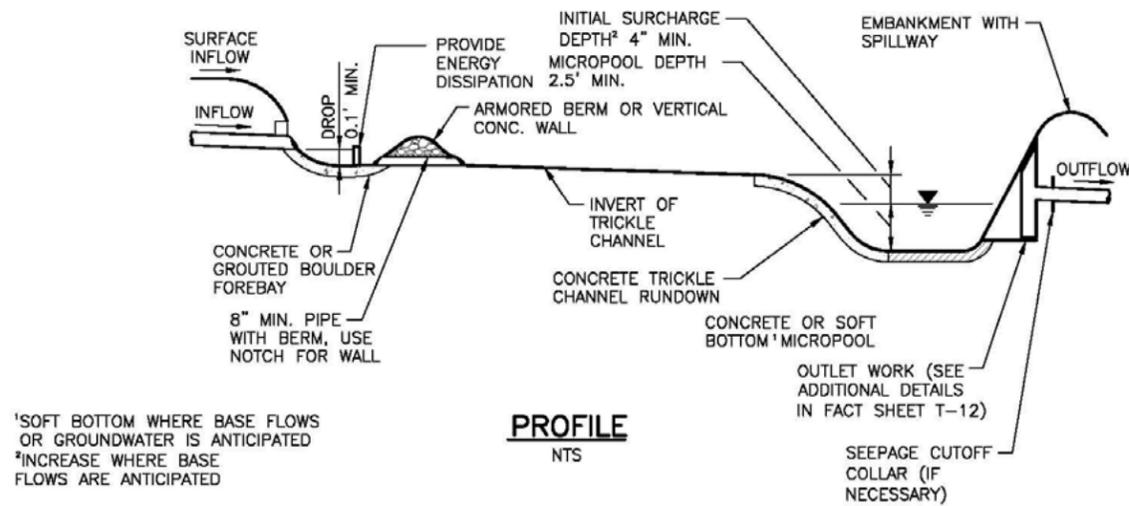
Figure 4-11. Detention Basin Details (from UDFCD Criteria Manual Vol. 3)
