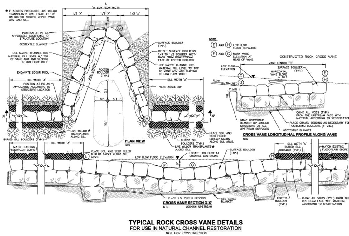
Figure 4-2. Rock Cross Vane Details
