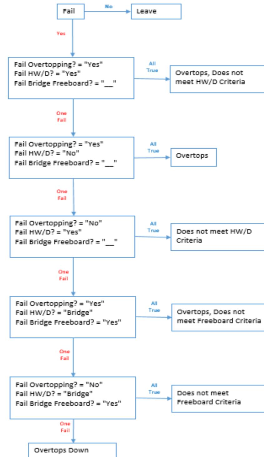
Figure 7-17. Bridge and Culvert Failure Analysis
