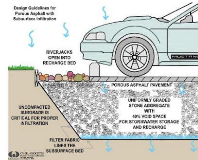
Figure 7-21. Pervious Pavements
