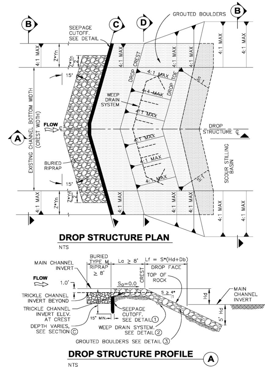
Figure 4-5. Drop Structure Details
