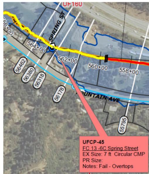
Figure 7-18. Example of Failing Structure
