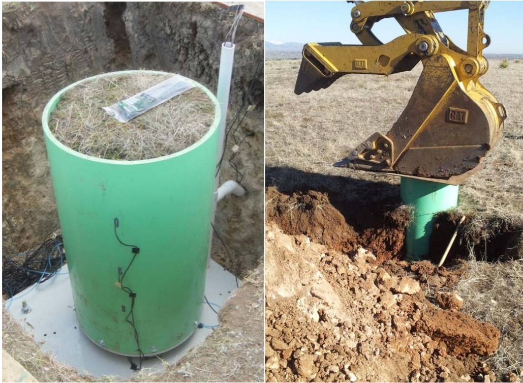
Figure 7 – Sterling Ranch Lysimeter and Soil Core Extraction
