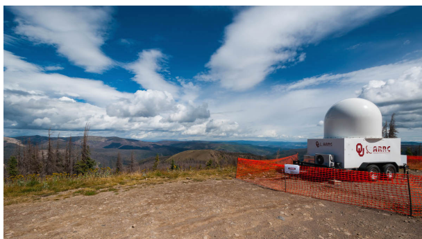
Fig. 3. The PX-1000 radar deployed at the Lobo Overlook of the Mineral County. The site was selected because of its altitude, which provide clear radar coverage toward the forest burned areas. The photograph is captured with a wide-angle lens, which show a 109^\circ field of view facing north. The radar is clear from blockages.
