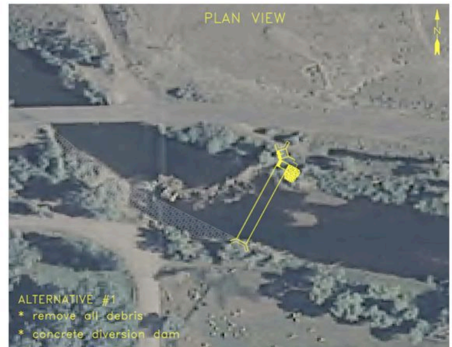
Figure 15. Proposed Design for Alternative 1: Concrete Diversion Dam
