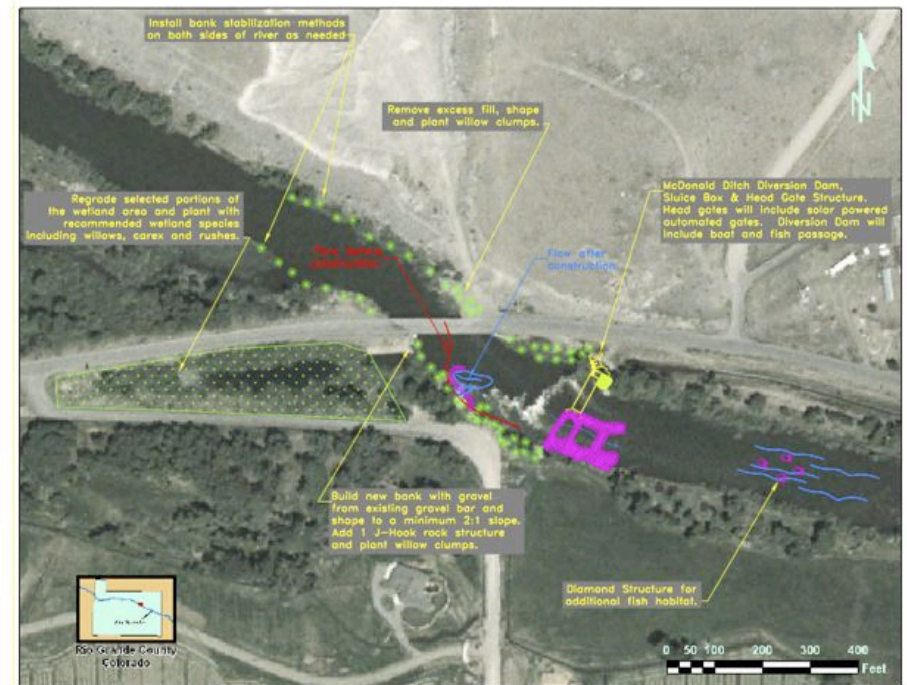
Figure 26. Selected Alternatives for the McDonald Ditch.
