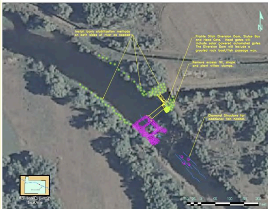
Figure 31. Selected Alternatives for the Prairie Ditch
